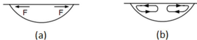
Figure 1.8: Weld pool convection due to negative surface tension gradient.
