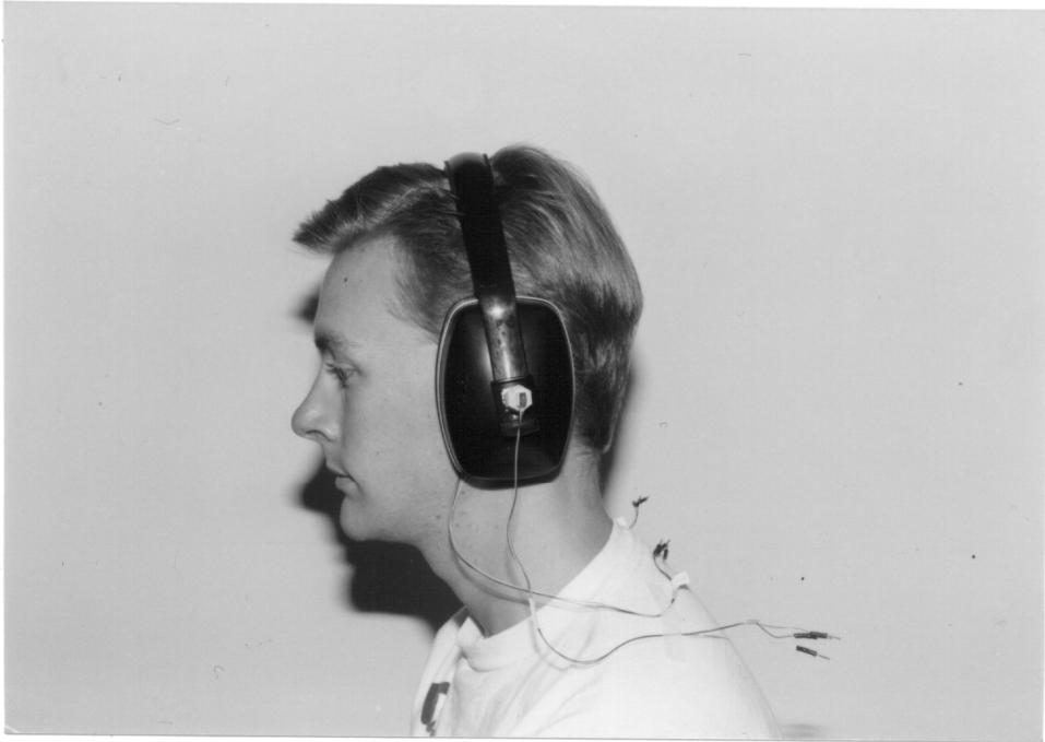
Figure 29. Knowles miniature microphone on the earmuff's exterior.
