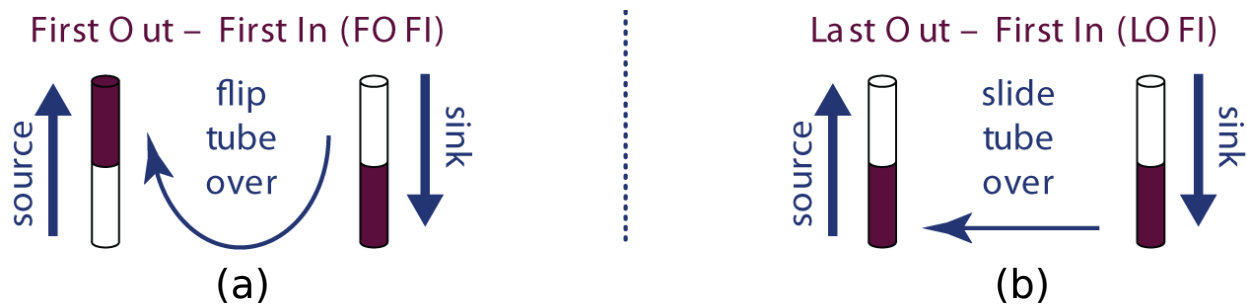
Figure 3.7: “First Out, First In” and “Last Out, First In” method to transport extracted fluid from a source to a sink for reinjection.
