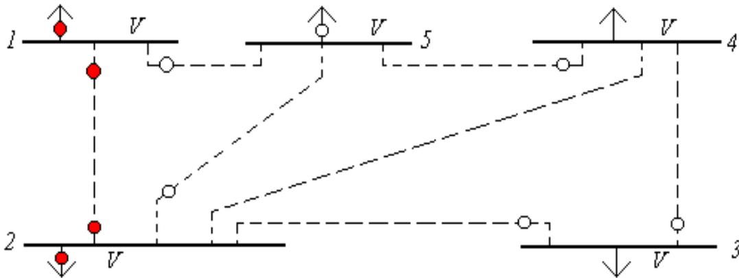
*Figure 2.3. IEEE Standard 5-Bus System with Topology Error*
