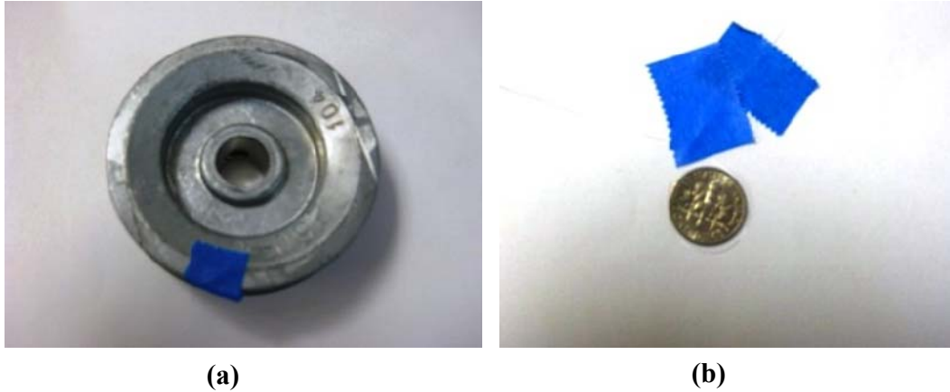
Figure 3.6 (a) The bare fibers wound around a pulley and (b) The fibers with different de-coating length as compared to a dime.
