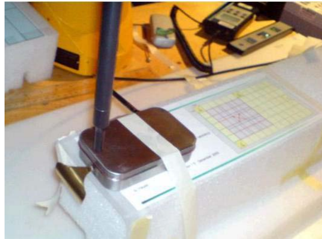
Figure 5.30 Picture of near-field measurement setup using DASY3™ system [SPEAG, 2006]. Near-field measurements were performed by Dr. Minh-Chau Huynh, Sony Ericsson.
