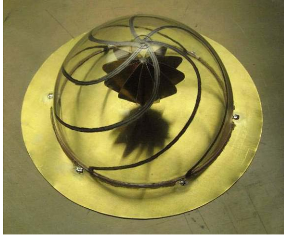
Figure 6.26 Picture of the multi-functional compact antenna prototype for SDR applications.
