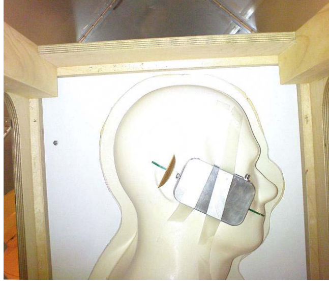
Figure 5.43 Picture of SAR measurement with DASY4™ system [SPEAG, 2007] with spoon UWB antenna in the cheek mode. Near-field measurements were performed by Dr. Minh-Chau Huynh, Sony Ericsson.
