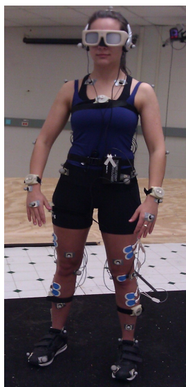
Figure 3.6 A participant with completed markers, EMG electrodes, and PLATO
