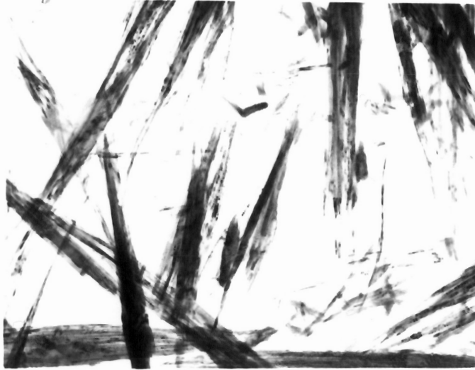
a) EDTA at 80 minutes - \gamma -FeOOH
