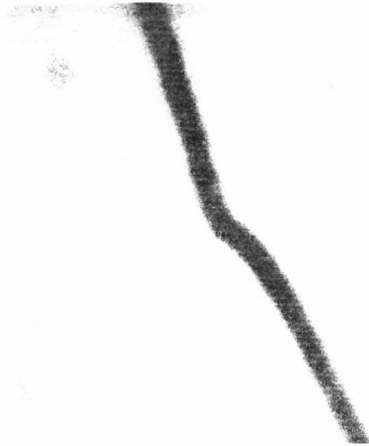
Fig.5.7 (a) A poly-Si grain boundary in the SEM picture and (b) the boundary as seen in EBIC
