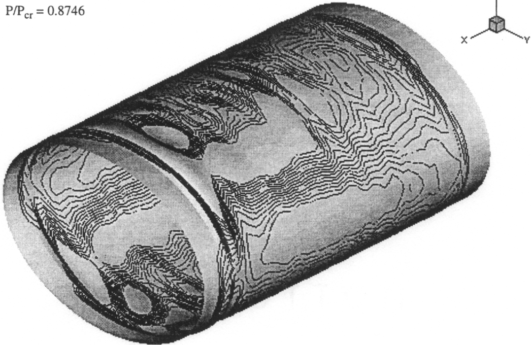
Figure 6-40 Deformed Shapes of the Perfect and Imperfect ( \pm 45/0/90 )s Cylinder with b/a = 0.70 .
