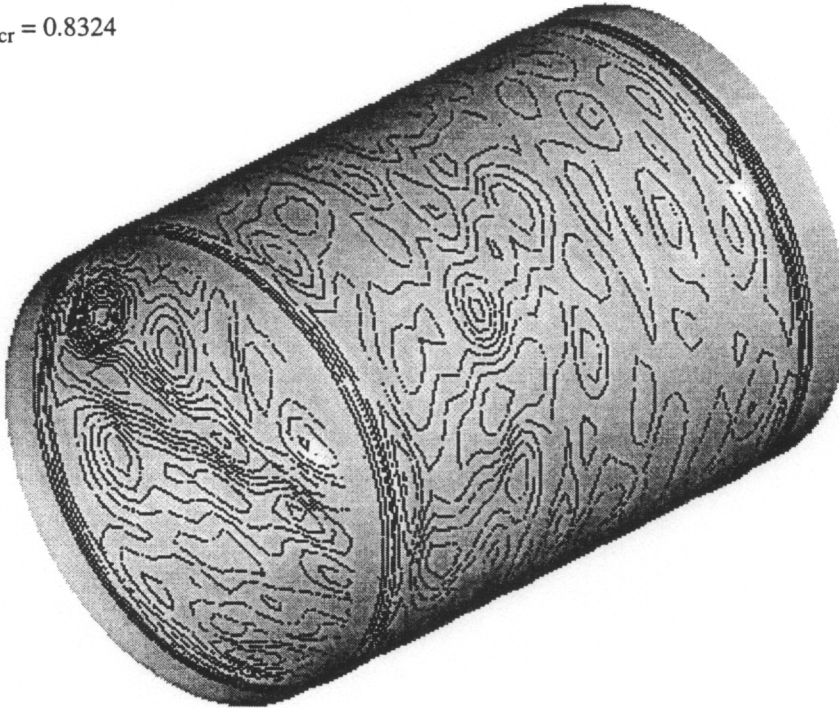
Figure 6-42 Deformed Shapes of the Perfect and Imperfect ( \pm 45/0/90 )s Cylinder with b/a = 1.00 .
