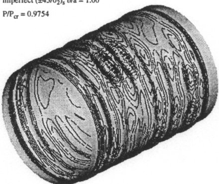
Figure C-12 Deformed Shapes of the Perfect and Imperfect (\pm 45/0_2)_s and (\pm 45/90_2)_s Cylinders with b/a = 0.85 and 1.00 .
