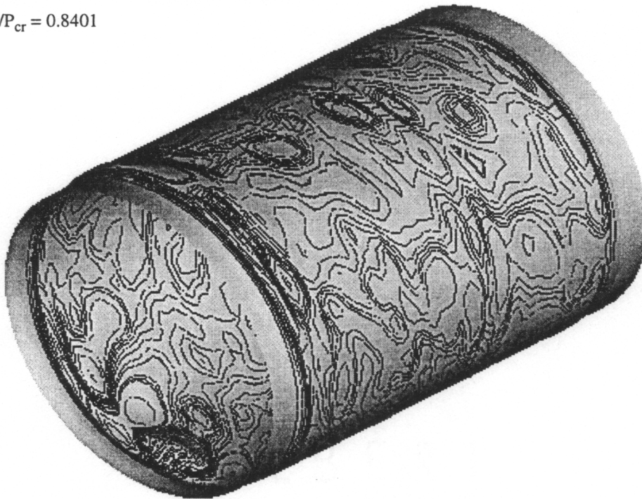
Figure 6-41 Deformed Shapes of the Perfect and Imperfect ( \pm 45/0/90 ) s Cylinder with b/a = 0.85 .
