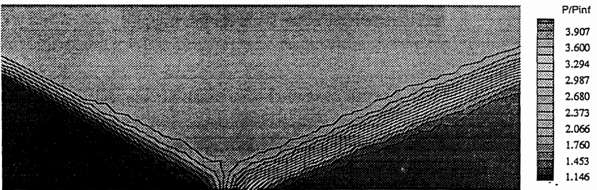
c – Static pressure contours, k_i = 1
