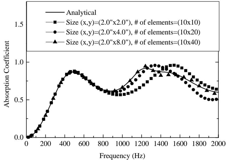
Figure 4.19: Comparison of normal incidence absorption coefficient as determined by analytical and finite element methods.
