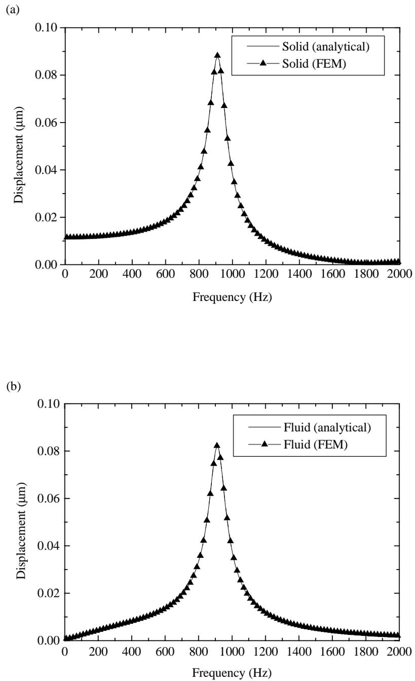
Figure 4.8: Surface displacement of Glass Wool due to mechanical force. A comparison of analytical and FEM results.
