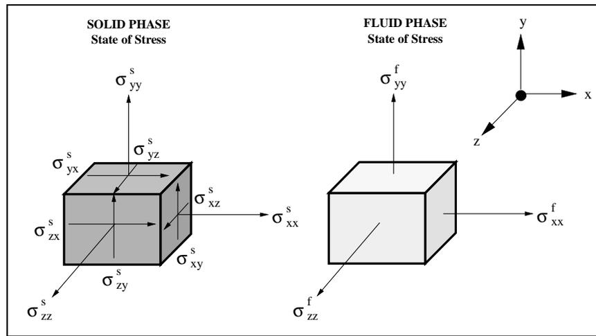
Figure 4.2 State of stress in the solid and fluid phases of an elementary macroscopic volume of porous material.
