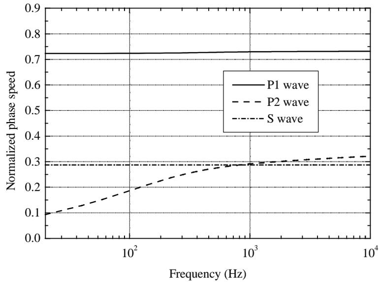
Figure 4.3(a): Variation of the normalized phase speed of the P1, P2 and S waves propagating in acoustic foam with respect to frequency.
