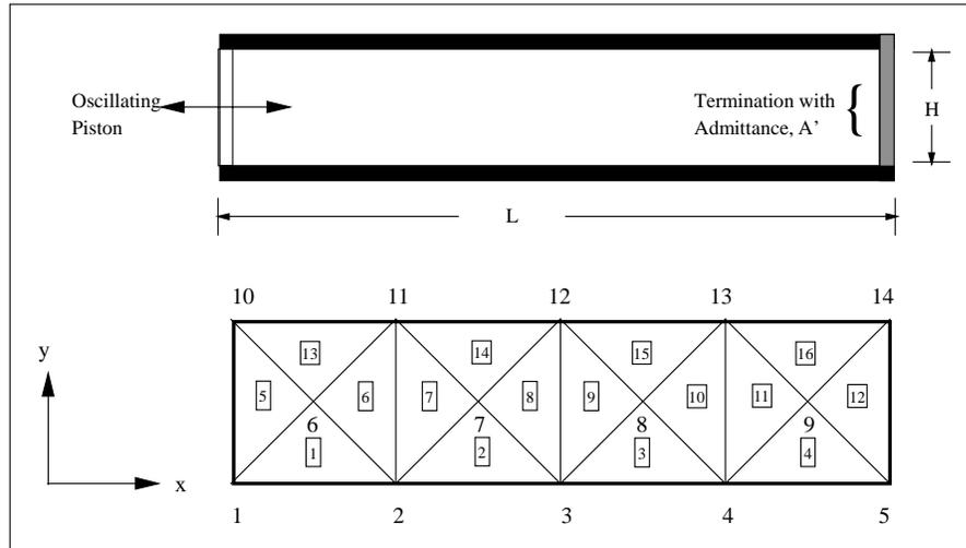
Figure 4.10: Illustration of a problem solved using numerical acoustic model and sample finite element mesh of the system.
