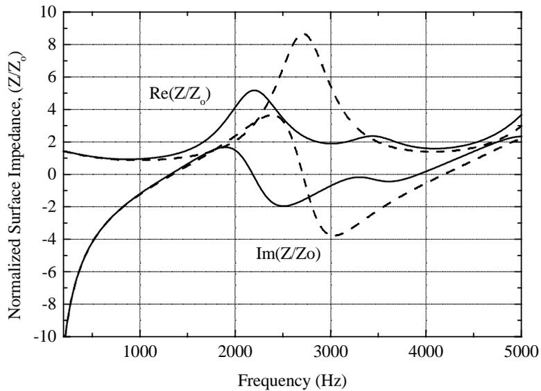
Figure 4.5(b): Normalized surface impedance vs. frequency of acoustic foam. The thickness of the layer is 2.0 cm. Normalized impedance of acoustic foam: ———. Normalized impedance of similar rigid framed material: - - - - -.
