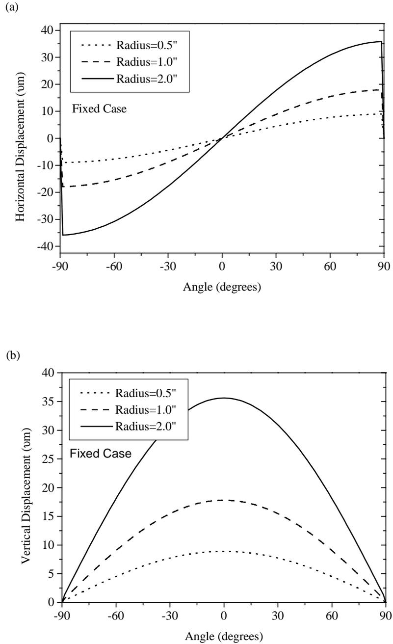
Figure 4.15(a): Horizontal displacement of PVDF actuator with “fixed” boundary conditions at 250 Hz with 300 V rms excitation. (b) Vertical displacement of PVDF actuator with “free” boundary conditions at 250 Hz with 300 V rms excitation.
