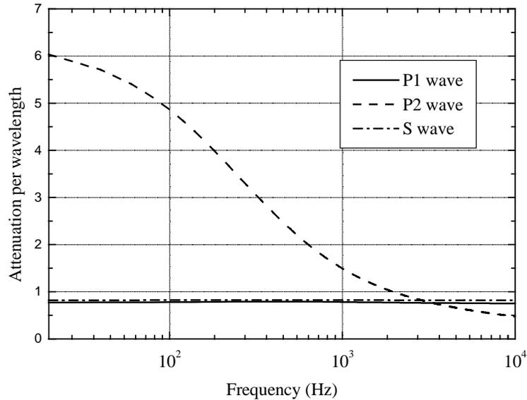
Figure 4.3(b): Variation of the attenuation coefficient of the P1, P2 and S waves propagating in acoustic foam with respect to frequency.
