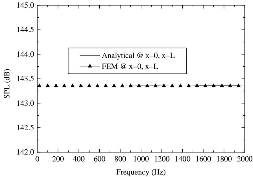
Figure 4.12: Verification of FEM model of acoustic system. Average SPL at  $x=0$  and  $x=L$  vs. frequency for rigid air-filled duct with anechoic termination excited by an oscillating piston.
