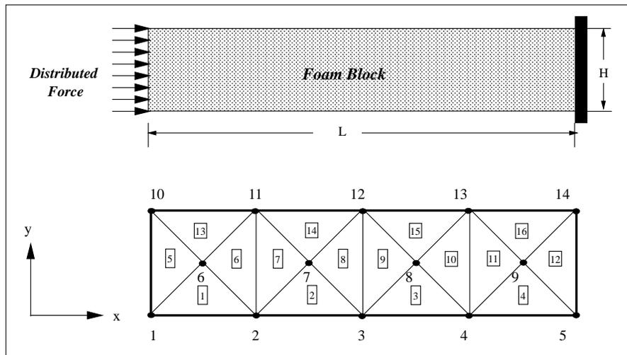
Figure 4.7: Illustration of a problem solved using numerical poroelastic model and sample finite element mesh of the system.
