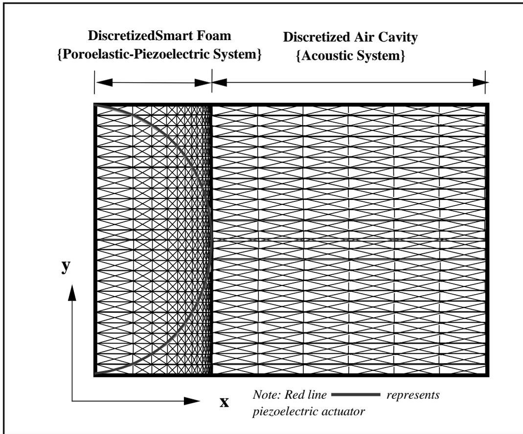
Figure 4.6. Illustration of *discretized* finite element model of smart foam in an air-filled duct.
