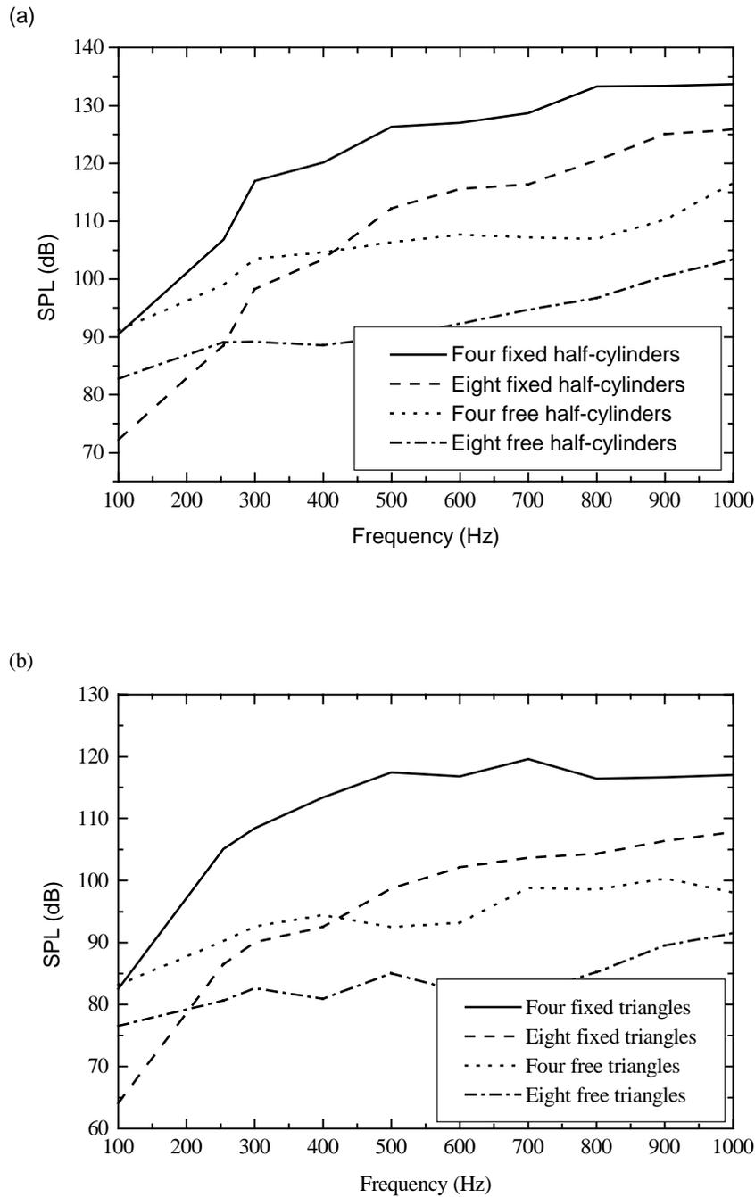
Figure 4.21: Sound pressure level vs. frequency generated by various smart foam array configurations excited at  $300 V_{\text{rms}}$  while positioned in rigid duct with anechoic termination (a) Smart foam with embedded PVDF shaped as half-cylinders (b) Smart foam with embedded PVDF shaped as triangles.
