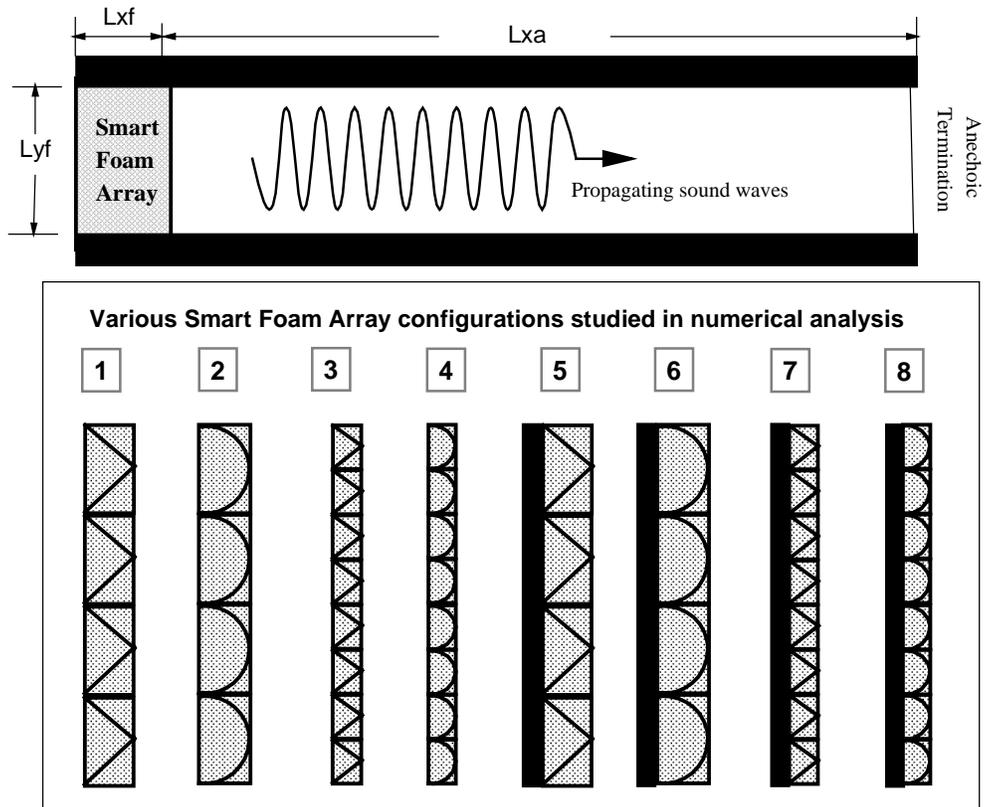
Figure 4.20 Illustration of smart foam actuator configurations investigated using the finite element approach : Smart foam with embedded PVDF shaped as (1) Four free triangles, (2) Four free half-cylinders (3) Eight free triangles, (4) Eight free half-cylinders, (5) Four fixed triangles, (6) Four fixed half-cylinders, (7) Eight fixed triangles, and (8) Eight fixed half-cylinders.
