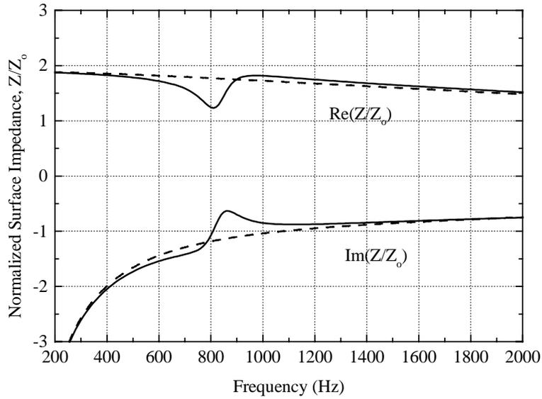
Figure 4.5(a): Normalized surface impedance vs. frequency of Glass wool. The thickness of the layer is 5.6 cm. Normalized impedance of glass wool: ———. Normalized impedance of similar rigid framed material: - - - - -.
