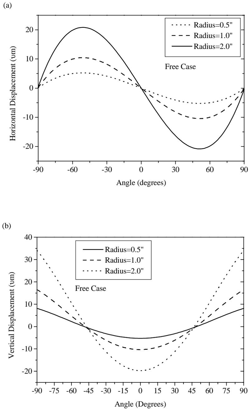
Figure 4.14(a): Horizontal displacement of PVDF actuator with “free” boundary conditions at 250 Hz with 300 V rms excitation. (b) Vertical displacement of PVDF actuator with “fixed” boundary conditions at 250 Hz with 300 V rms excitation.
