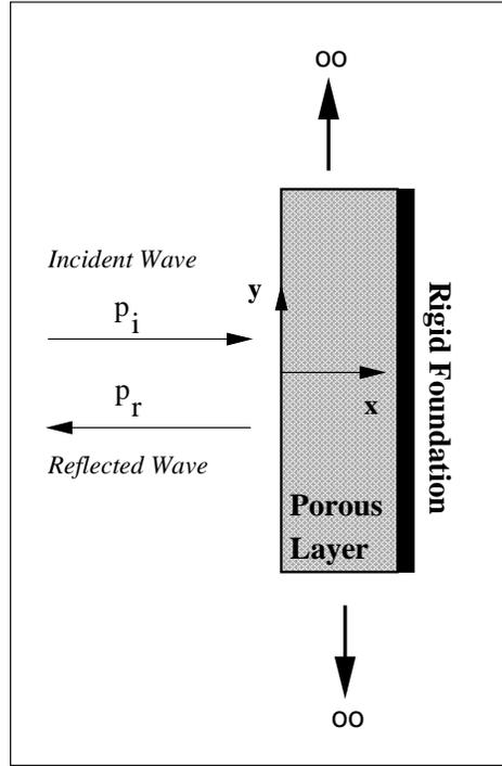
Figure 4.4 Illustration of a porous layer bonded to a rigid foundation and excited by a normal incident plane acoustic wave.
