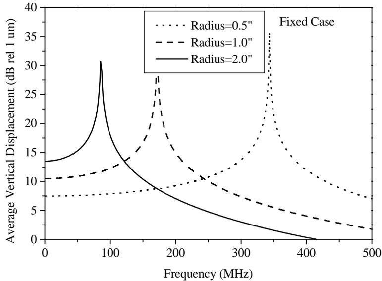
Figure 4.16: Average vertical displacement of PVDF actuator with “fixed” boundary conditions vs. frequency with  $300 \text{ V}_{\text{rms}}$  excitation.
