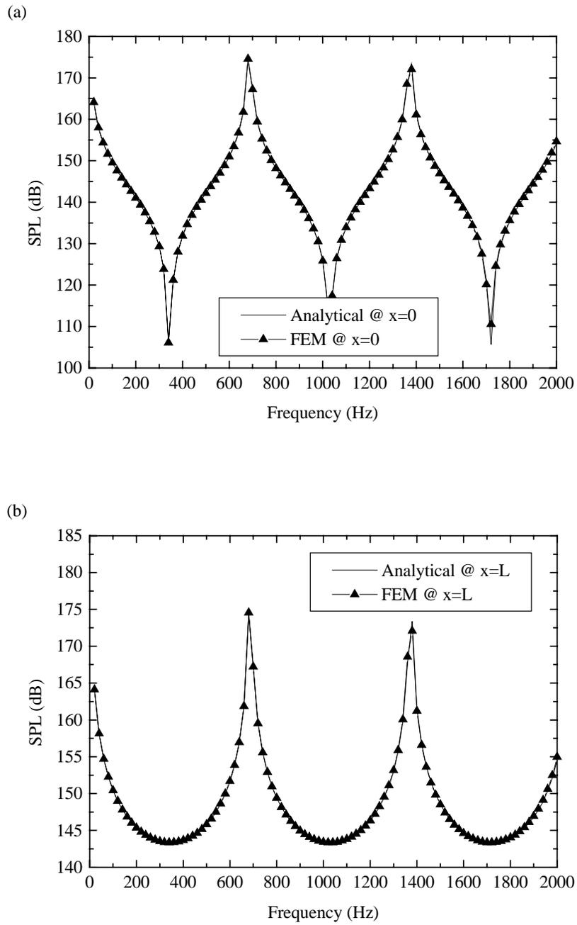
Figure 4.11: Verification of FEM model of acoustic system. Average SPL at  $x=0$  and  $x=L$  vs. frequency for rigid air-filled duct excited by an oscillating piston.
