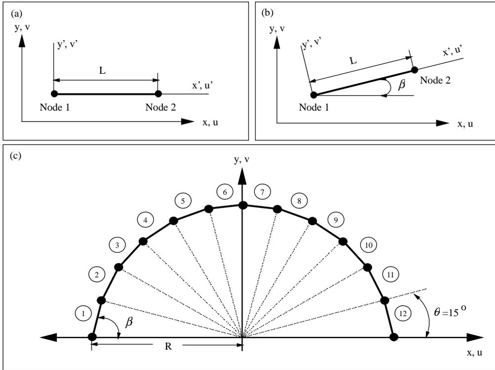
Figure 4.13(a): Piezoelectric finite element with one degree of freedom per node (b) Piezoelectric finite element with two degrees of freedom per node (c) Assembly of piezoelectric finite elements to establish cylindrical actuator of radius, R.
