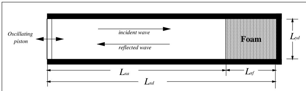
Figure 4.17: Illustration of acoustic waveguide terminated by a foam layer. Represents system used verify finite element acoustic-poroelastic coupling procedure.
