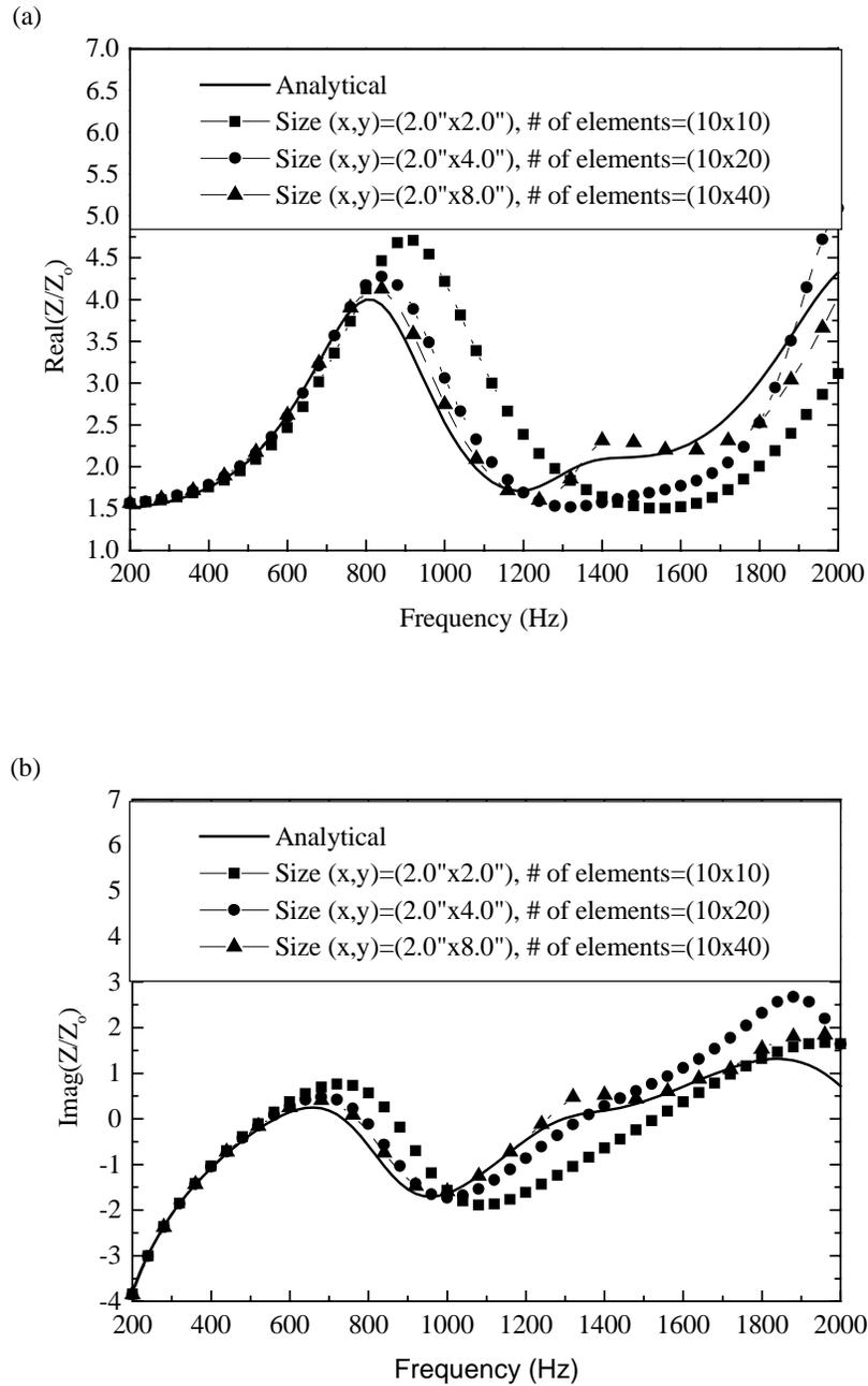
Figure 4.18: Comparison of normalized acoustic impedance as determined by analytical and finite element methods (a) Real part. (b) Imaginary part.
