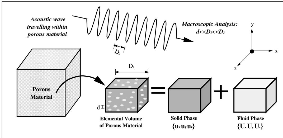
Figure 4.1 Illustration of a generic porous material and the macroscopic modeling approach.
