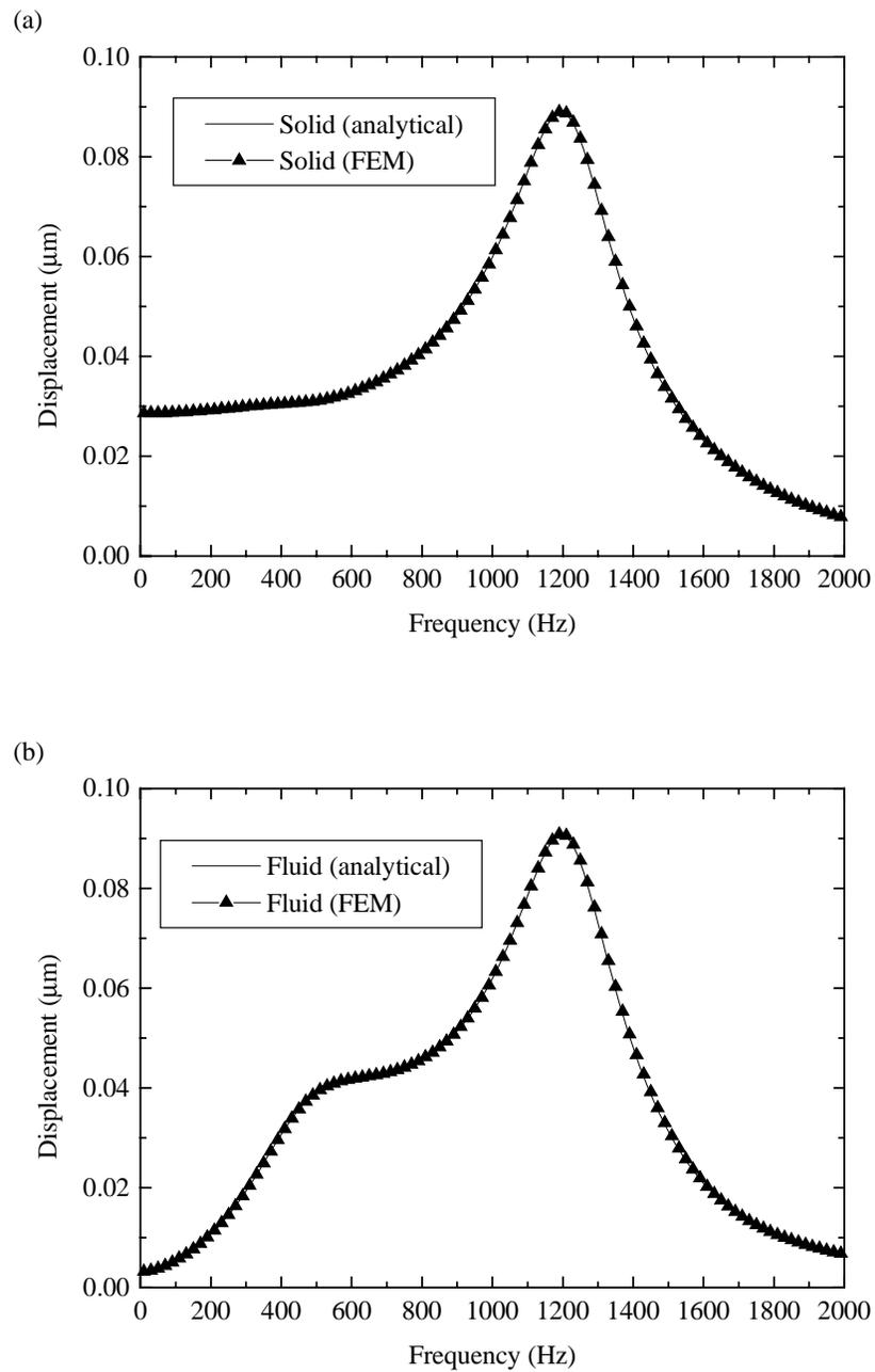
Figure 4.9: Surface displacement of partially-reticulated foam due to mechanical force. A comparison of analytical and FEM results
