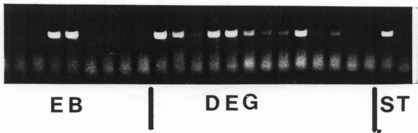
**Figure 2.** Sample gel showing detection of the WAPPC-3 transgene in blastocysts and degenerate embryos. EB, expanded blastocysts; DEG, degenerate embryos; ST, 100 and 10 genome copies of WAPPC-3 transgenic mouse DNA, respectively.
