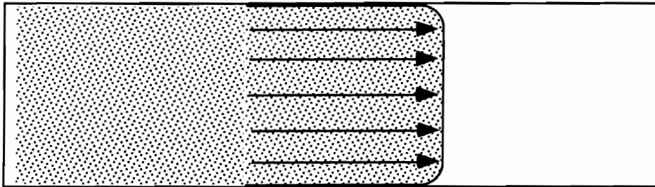
Bulk Flow arising from an Electroosmotically-driven system.
