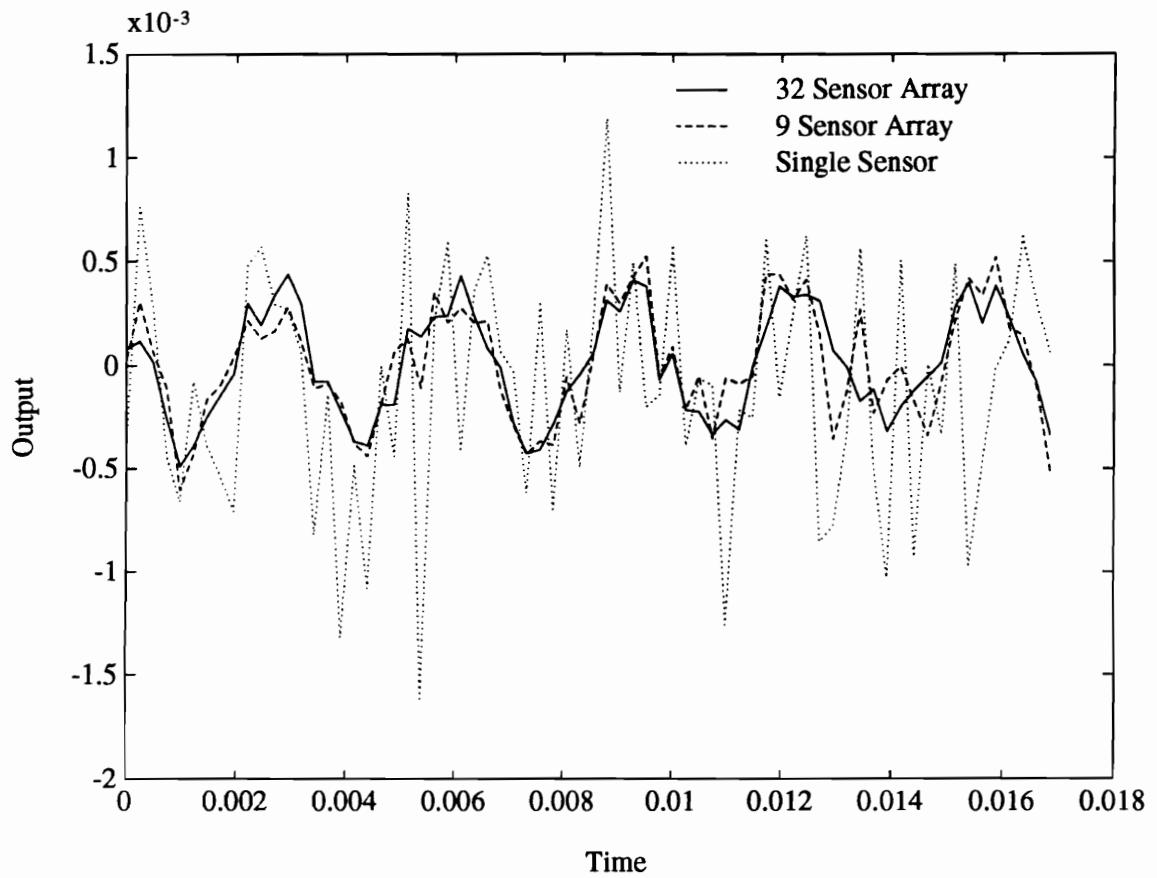
Figure 3.3: Simulated SNR Performance of 1, 9, and 32 Element Arrays – Time Domain
