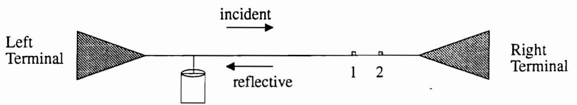
Figure C.1: Apparatus Setup To Measure Reflection Coefficient of Right Sandbox
