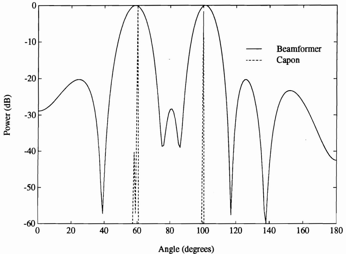
Figure 2.4: Power Output of Beamformer vs. Capon Estimator
