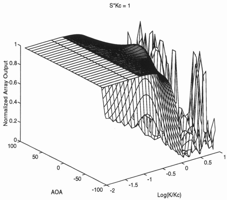
Figure 3.7: Normalized Output of 3x3 Array for Off Angle and/or Off Wavenumber Signals For  $k_c s = 1$
