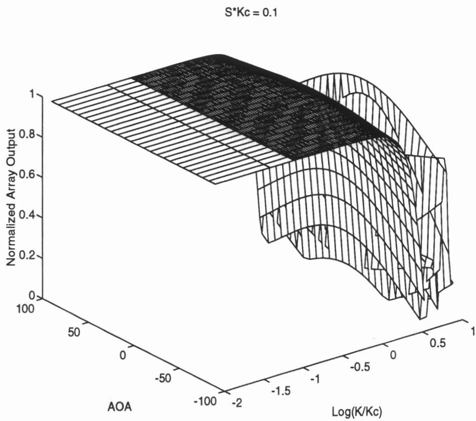
Figure 3.6: Normalized Output of 3x3 Array for Off Angle and/or Off Wavenumber Signals For  $k_c s = .1$
