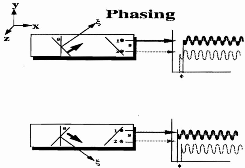
Figure 3.9: Determination of AOA from Phasing
