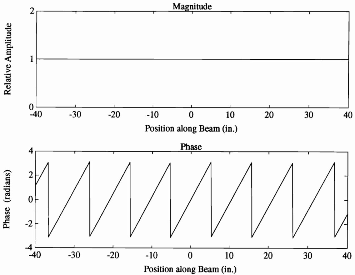
Figure 4.4: Theoretical Magnitude and Phase of Incident Wave Without Mass Discontinuity Located at  $x = 0$
