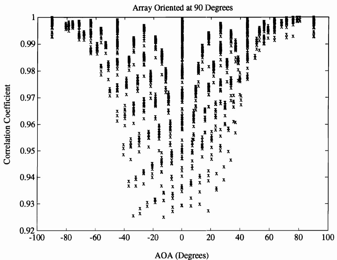
Figure 5.10: Correlation Coefficients for Array Positioned at 90 Degrees
