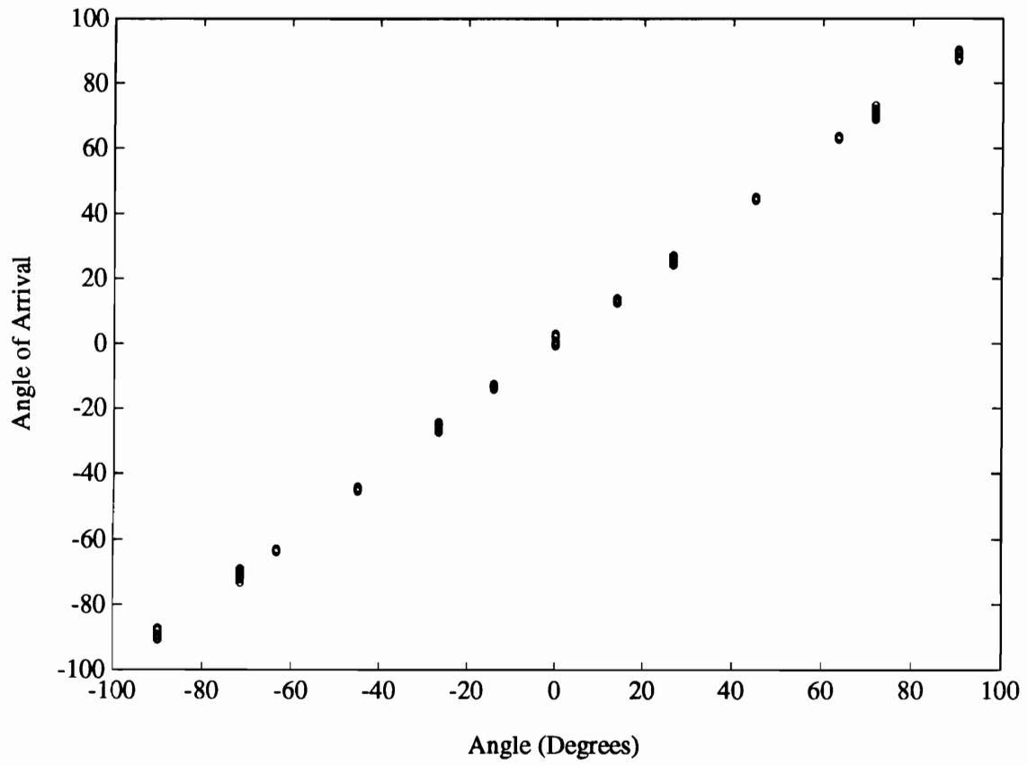
Figure 4.19: Experimentally Determined Angle of Arrival for Infinite Beam vs Angle of Arrival
