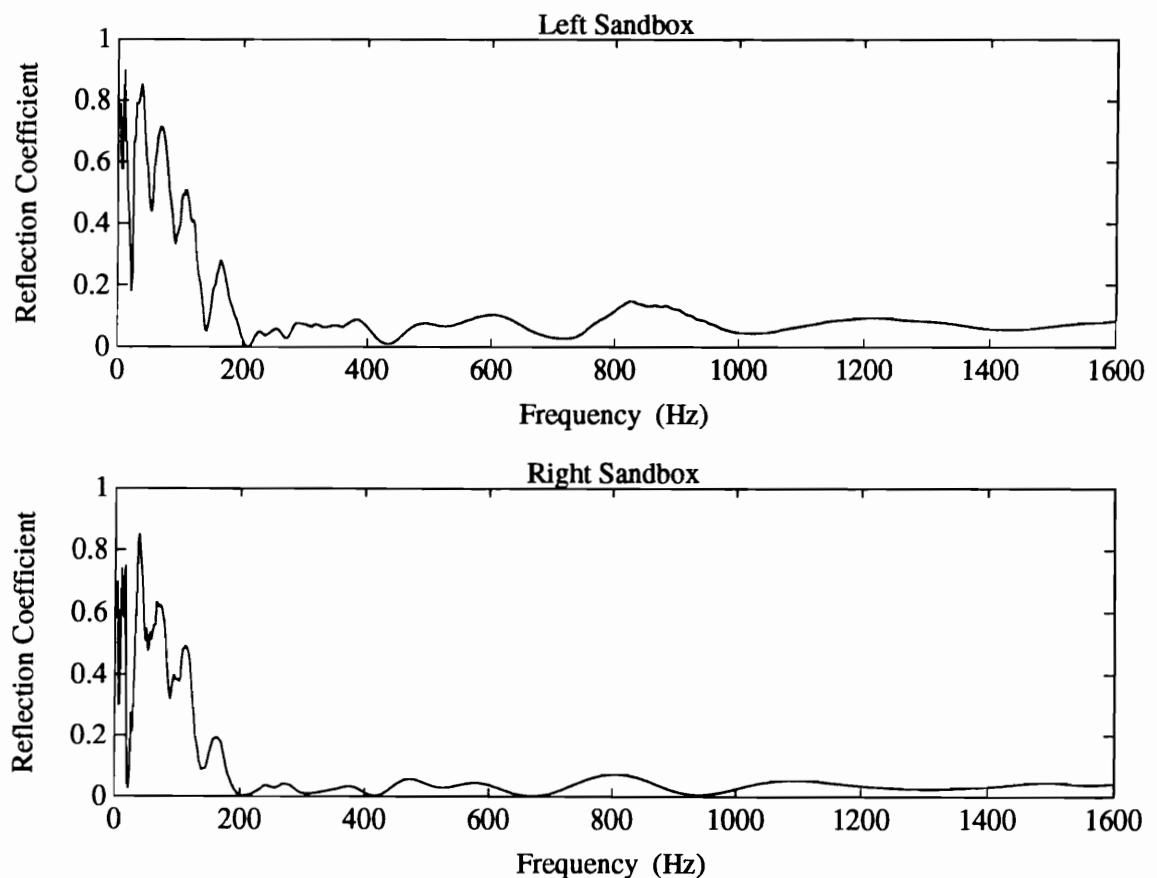
Figure 4.3: Reflection Coefficient of Sandboxes
