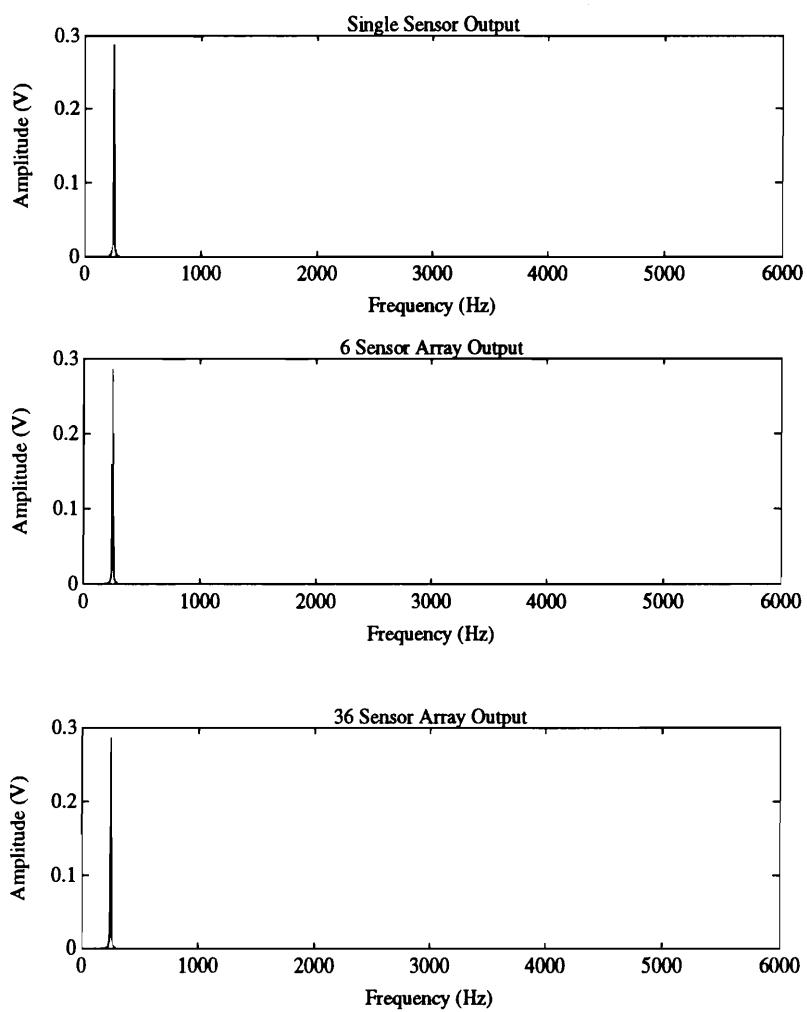
Figure 4.13: Frequency Response of Array – Autospectra
