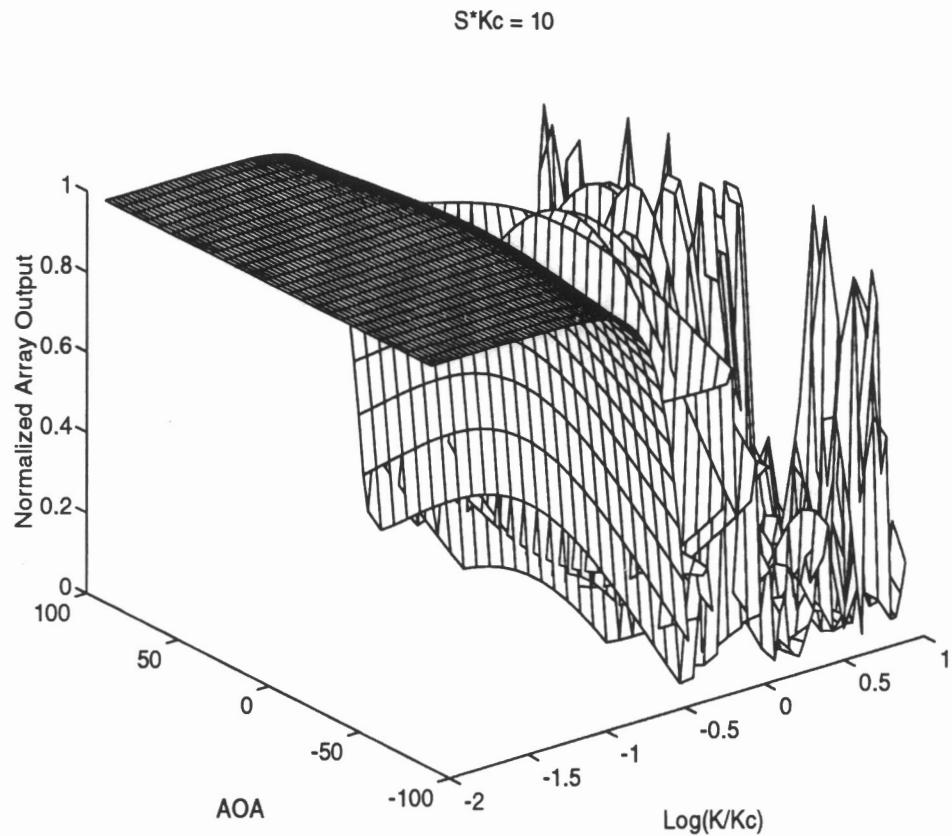
Figure 3.8: Normalized Output of 3x3 Array for Off Angle and/or Off Wavenumber Signals For  $k_c s = 10$
