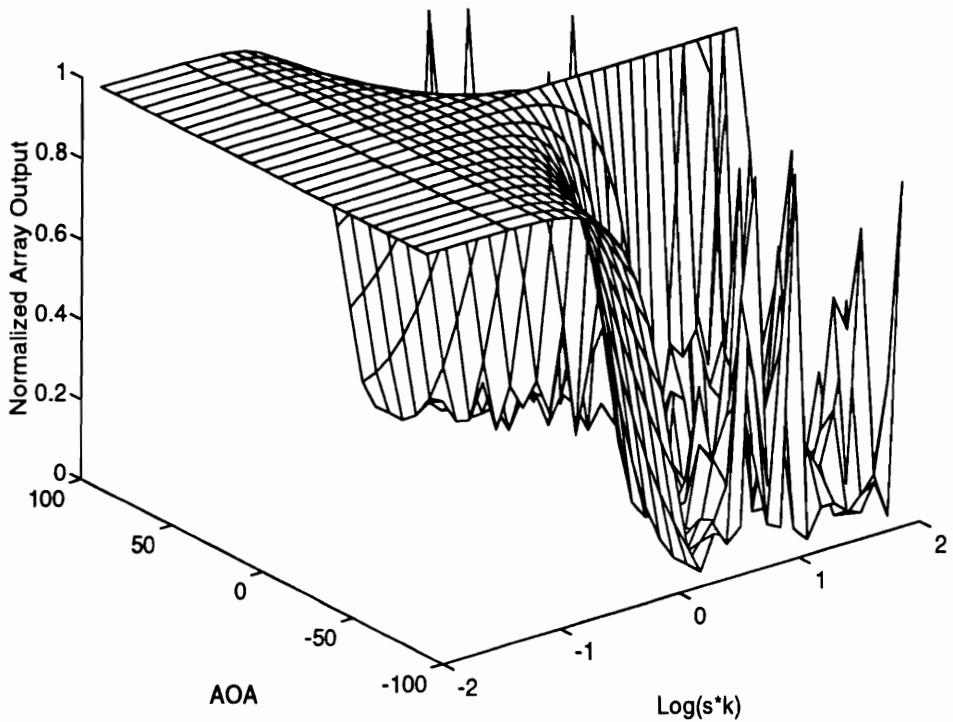
Figure 3.4: Normalized Output of 3x3 Array for off Angle Measurements – Array Tuned at 0 Degrees, Single Frequency
