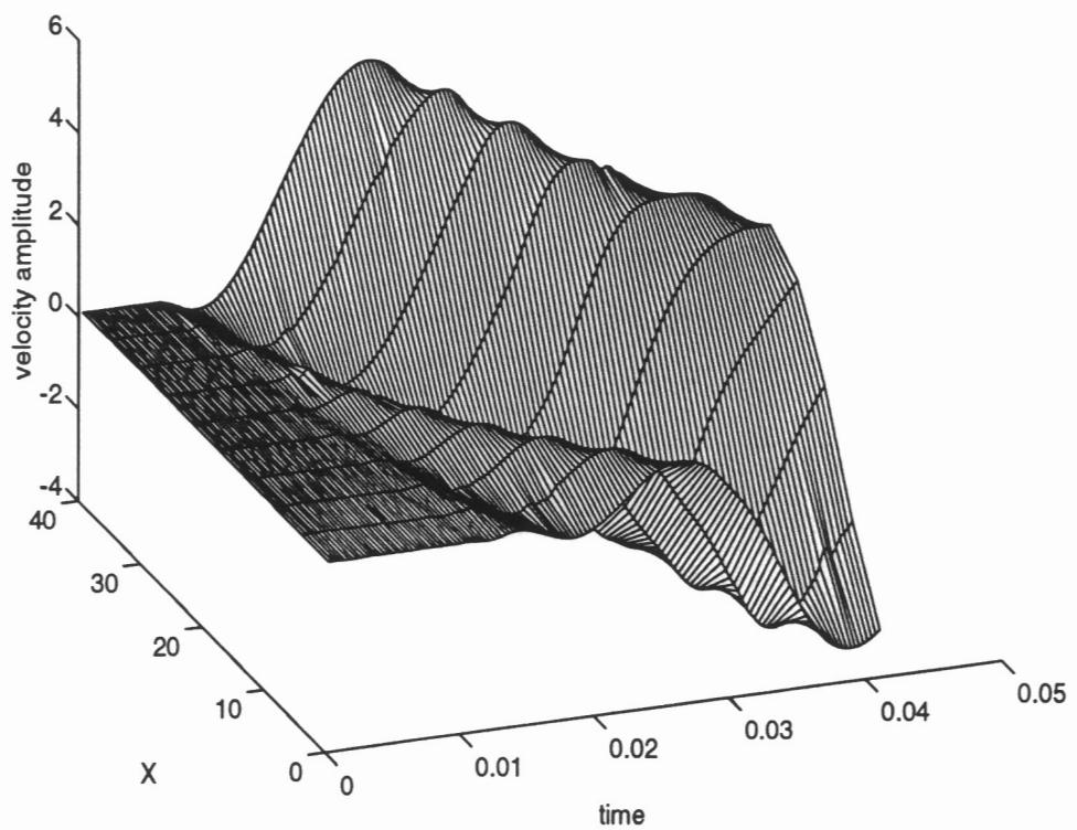
Figure 5.1: Example of Dispersion in Beam – Plot of Time History for Different Sensor Locations in Response to Impact
