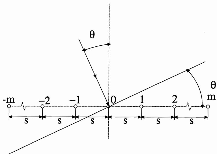
Figure 2.2: Angle of Arrival and Time Delay Schematic for Linear Array
