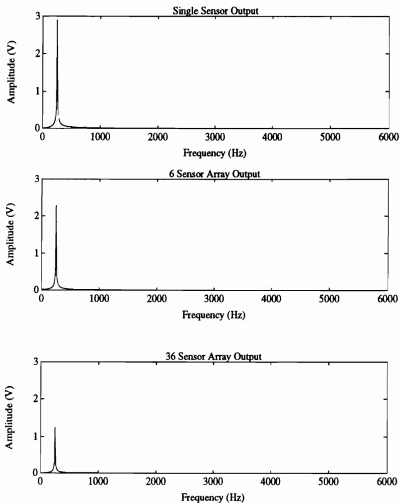
Figure 4.12: Frequency Response on nonbeamformed spectra
