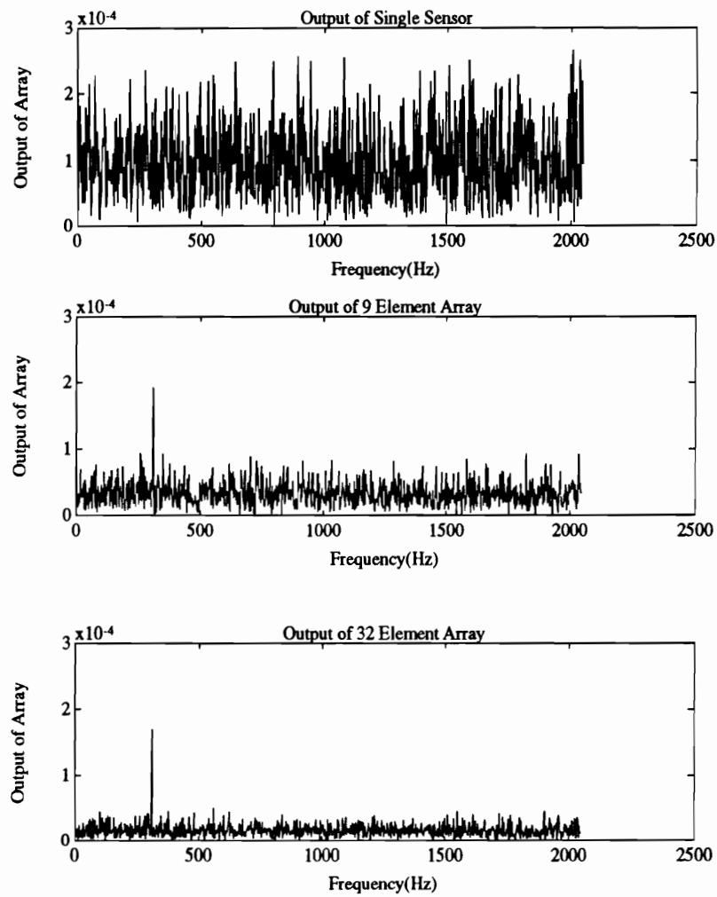
Figure 3.2: Simulated SNR Performance of 1, 9, and 32 Element Arrays – Frequency Domain
