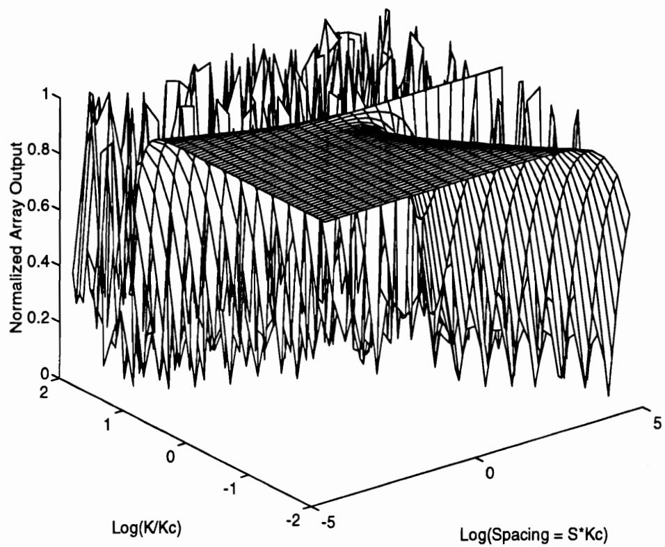
Figure 3.5: Normalized Output of 3x3 Array with Errors in Wavenumber
