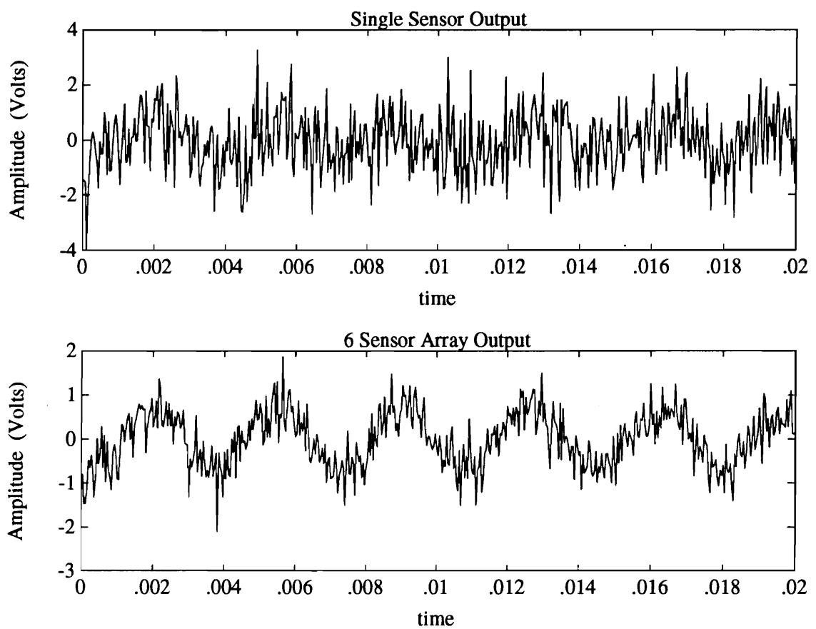
Figure 4.9: Time Domain Response of 6 Element Array – Beamformed
