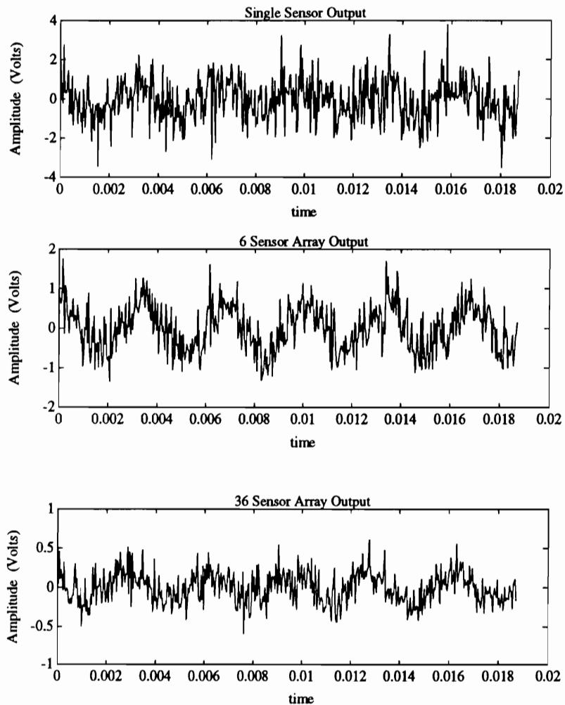
Figure 4.11: Time Domain Response of Infinite Beam Using Non-Beamformed Array
