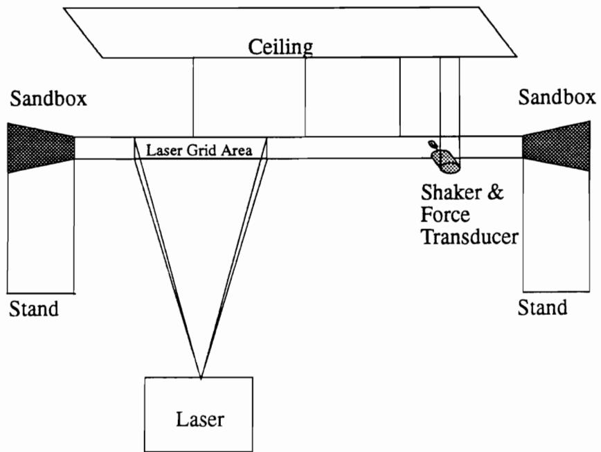
Figure 4.2: Experimental Setup Using Laser
