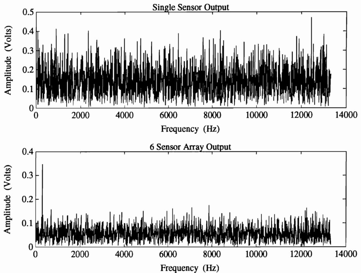
Figure 4.14: Frequency Domain Response of Infinite Beam Using Beamformed Array
