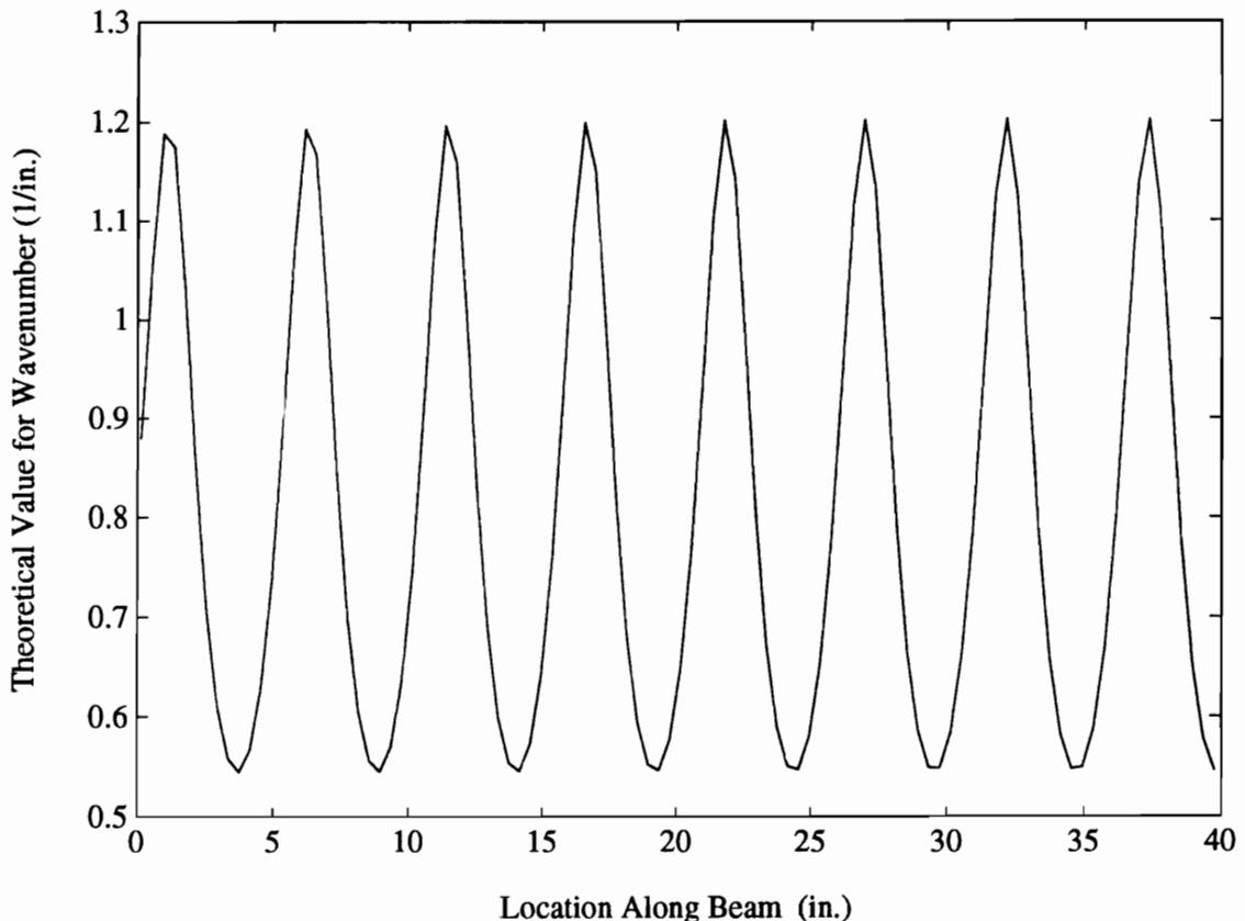
Note: This figure shows the estimation of  $k$  based on the instantaneous slope of the phase line. It depicts how a nonlinear phase causes variations in the estimation of  $k$ .
