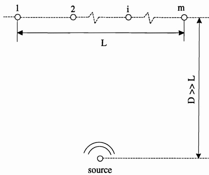
Figure 2.1: Schematic of Simple Linear Array
