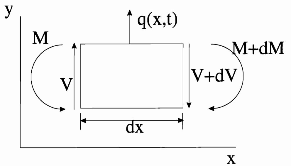
Figure A.1: Free Body Diagram of Differential Element of Beam
