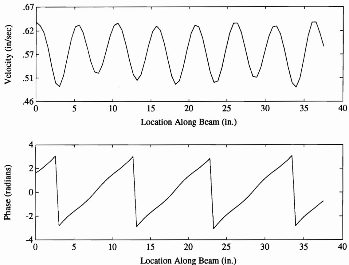
Figure 4.7: Experimental Verification of Beam Displacements with 10% Reflections
