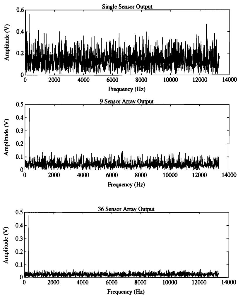
Figure 4.15: Frequency Response of Larger Arrays – Beamformed
