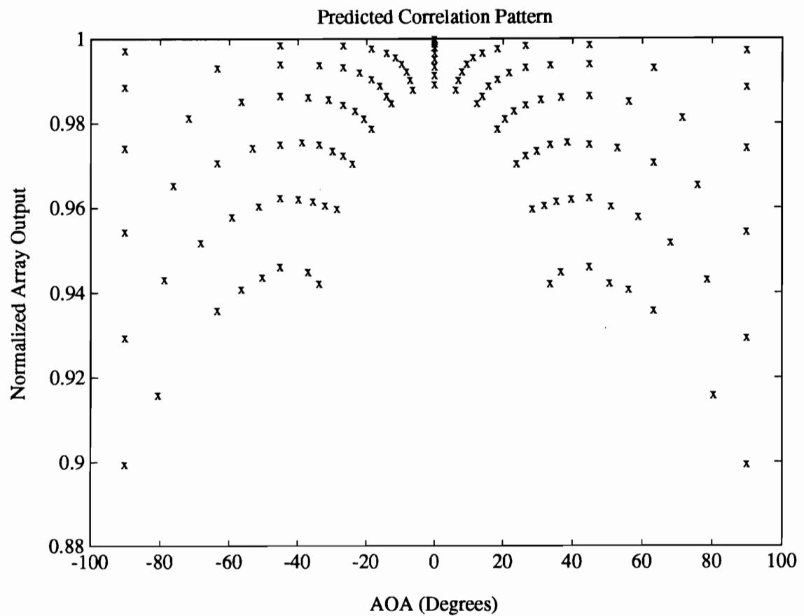
Figure 5.5: Correlation Prediction Based on Beampattern Response
