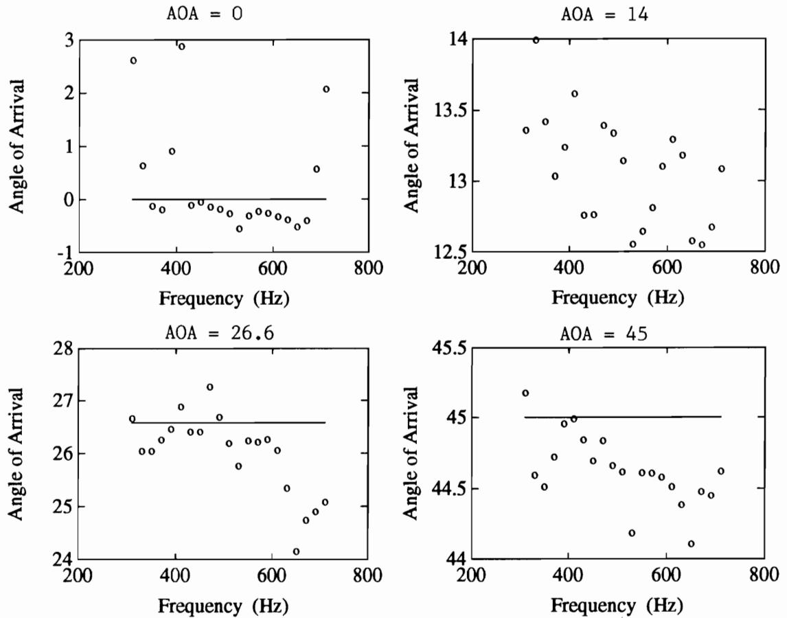
Figure 4.17: Experimentally Determined Angle of Arrival for Infinite Beam
