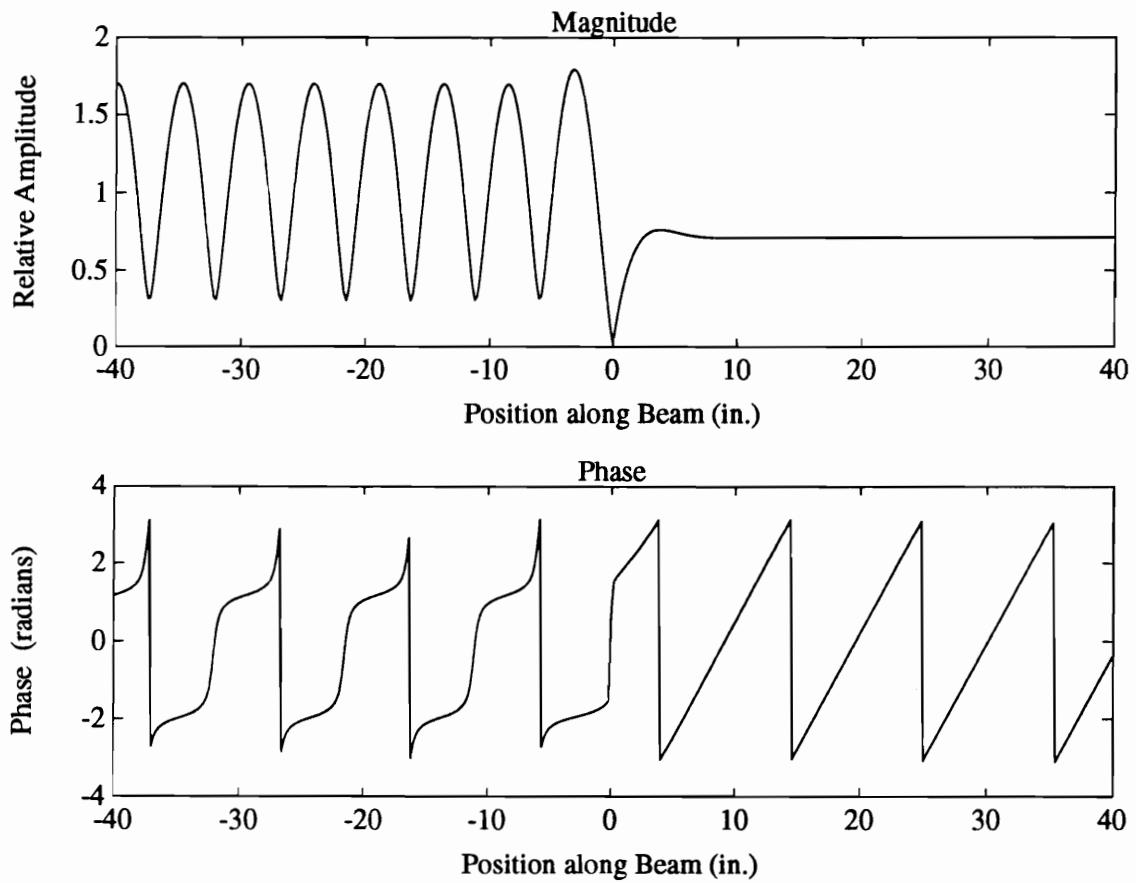
Figure 4.5: Theoretical Magnitude and Phase of Incident Wave With Mass Discontinuity
