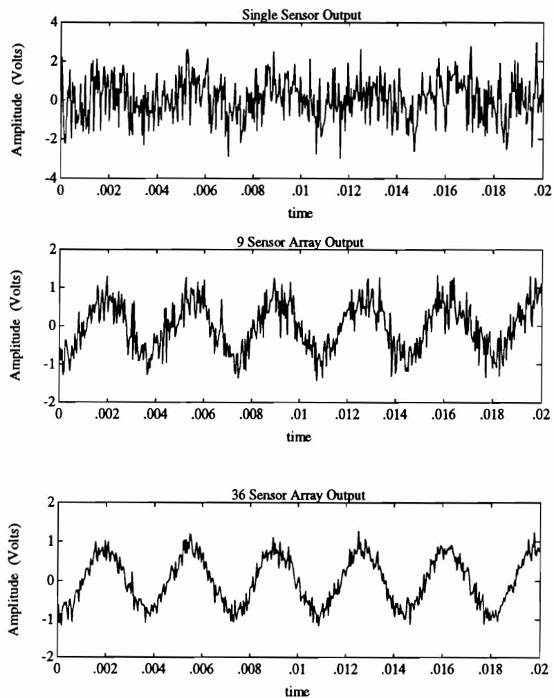
Figure 4.10: Time Domain Response of Infinite Beam Using Beamformed Array
