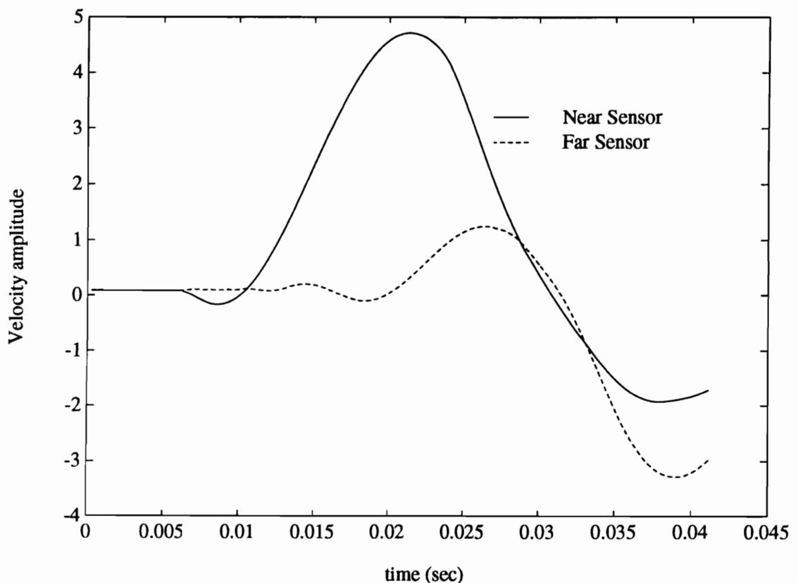
Figure 5.2: Time Histories at Two Different Beam Positions in Response to Impact
