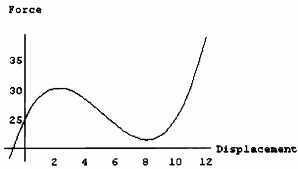
Figure 3.3. Force-displacement relation for a nonlinear nonmonotonic spring.
