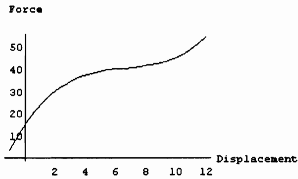
Figure 3.2. Force-displacement relation for a nonlinear monotonic spring.
