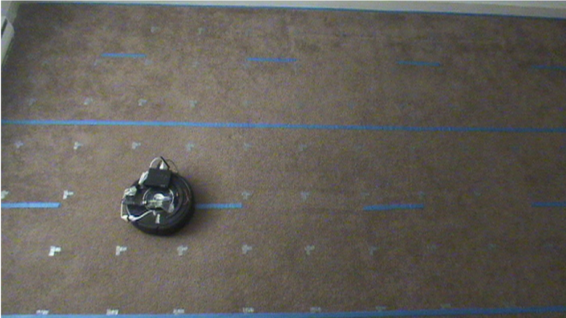
Figure A.2: An overhead view of the evading agent in the middle of its lane. The blue tape represents the counter-flow lanes that make up the road. The gray tape is the grid used to calibrate the Cricket measurement system.
