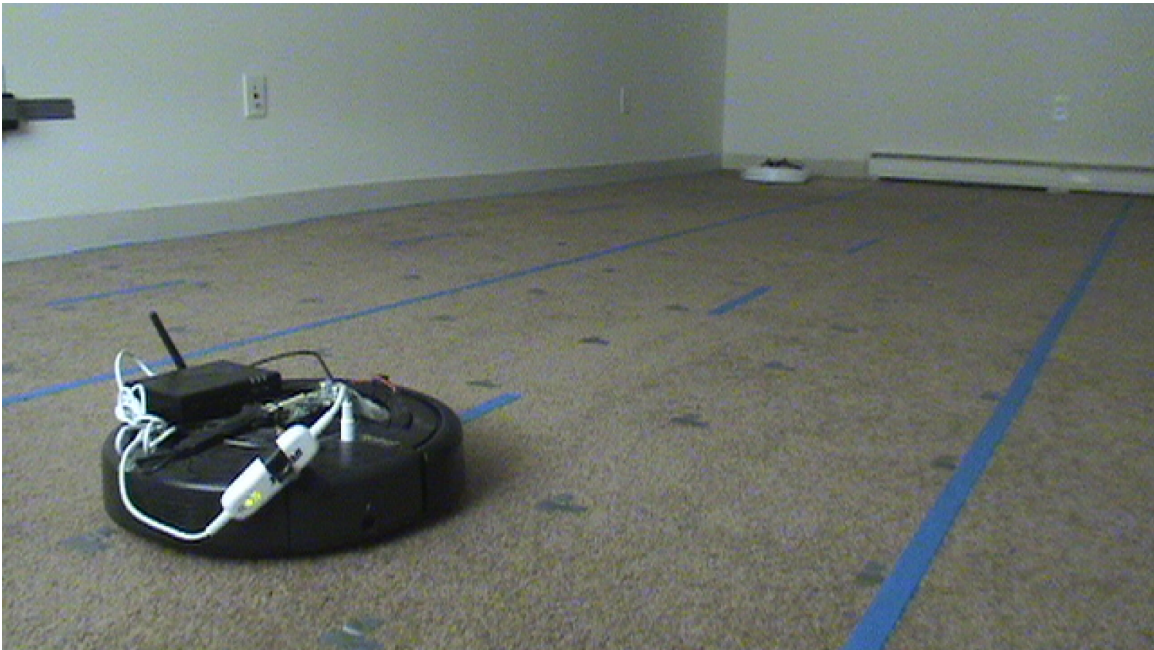
Figure A.1: Start of a scenario. Each agent is placed in opposite corners of the room. Each agent is equipped with a FitPC2 mounted with velcro and a listener Cricket module mounted to the top of the Roomba. The robot and processor were interfaced via the IRobot serial connection.
