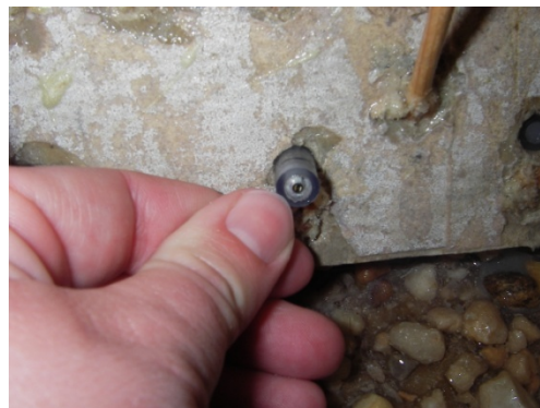
Figure 2.1. Miniature constant temperature anemometer probe being inserted into the model streambank (Dantec MiniCTA flush mounted hot-film probe 55R46).
