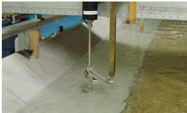
Figure 2.2. Sontek 16 MHz Side-looking MicroADV (acoustic Doppler velocimeter).
