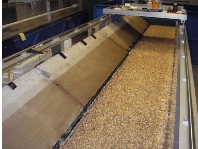
Figure 3.4. Streambank geometry constructed of masonry board hinged at the bank toe to provide sensor access for the hot-film probe.
