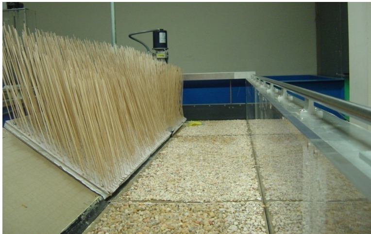
Figure 3.7. Shrub bank panel.
