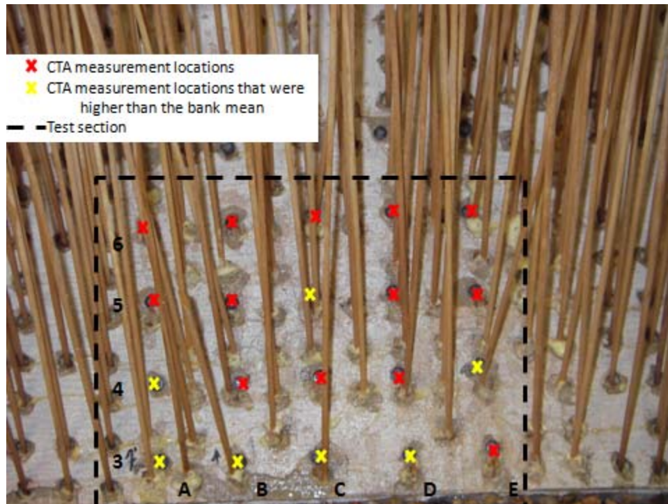
Figure 5.4. Location of hot-film anemometer measurements of boundary shear stress in reference to the shrub dowel location for 5 cross-sections (A-E). Locations where BSS was greater than the bank median are highlighted with yellow symbols.
