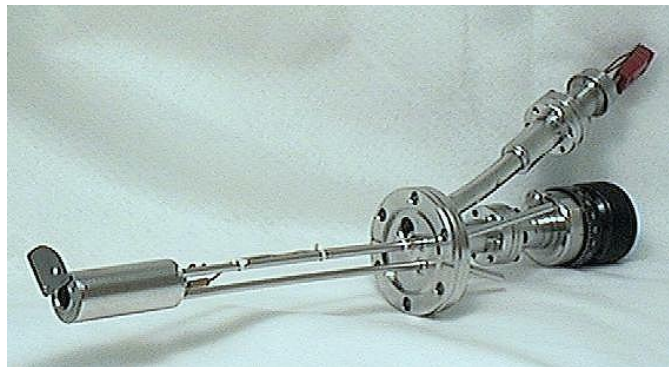
Figure 2.4: Crucible Style Evaporator used for the high vacuum deposition of fullerene films.
