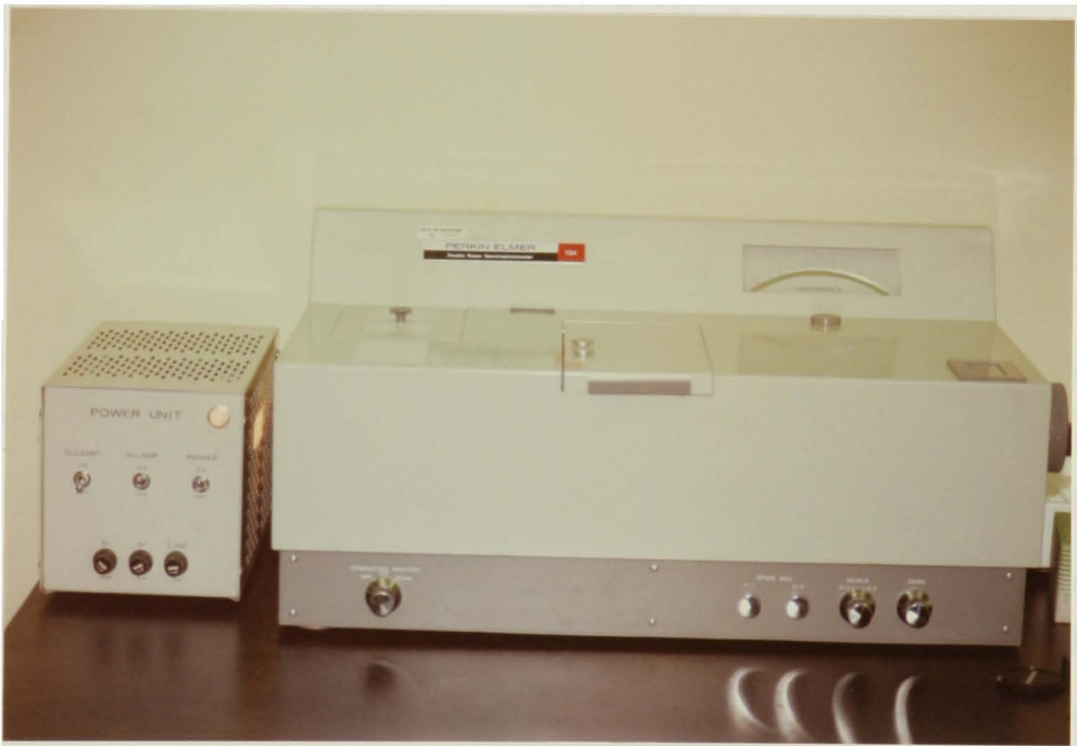
Fig. 18. (a) Apple leaf with discs removed for measuring the total chlorophyll content per unit-leaf area. (b) a double beam spectrophotometer.
