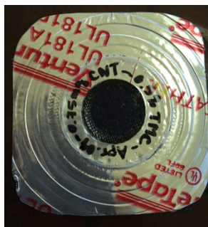
Figure 7-3. Picture of a CNT membrane masked with aluminum tape for testing inside the water permeation setup.
