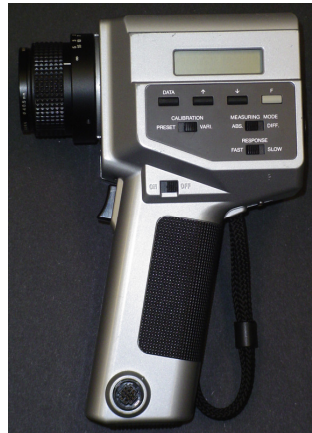
Figure 3.8 A photometer (Minolta CS-100)
