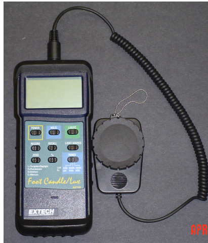
Figure 3.6 A light meter (Extech – Model 407026)
