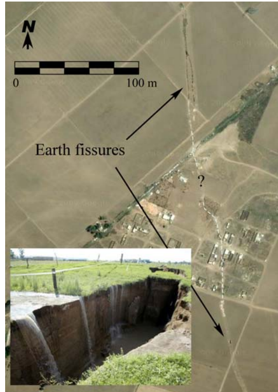
Figure 4.1. Aerial view of the most spectacular fissure of the Tesistan valley, Mexico. The dashed white line in the aerial photograph indicates the inferred location of the fissure on the land surface. The photograph in the lower left shows the affect of piping that increased the size of this fissure after a heavy rain.
