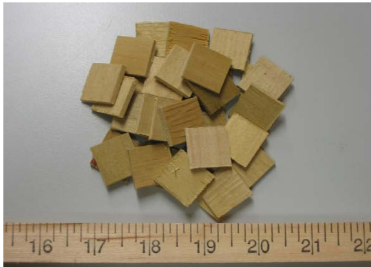
Figure 3.2 Yellow-poplar chips used in steam explosion
