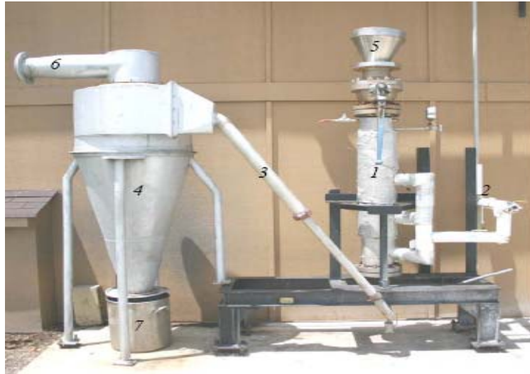
Figure 3.3 Steam explosion batch reactor used in this study
