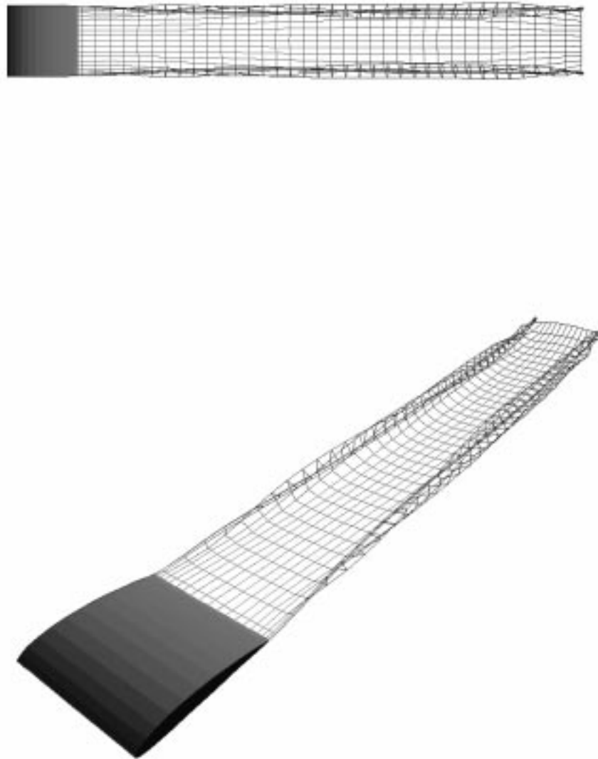
Figure 2.39: Flow Over A ClarkY Airfoil (AR=1.0) Out of Ground Effect; Doublet Panel Method
