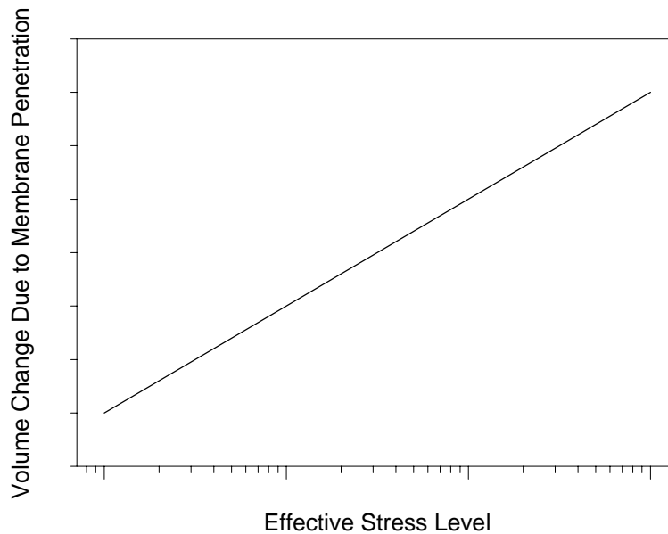
Figure 4.18 - Relationship Between Membrane Penetration and Effective Stress
