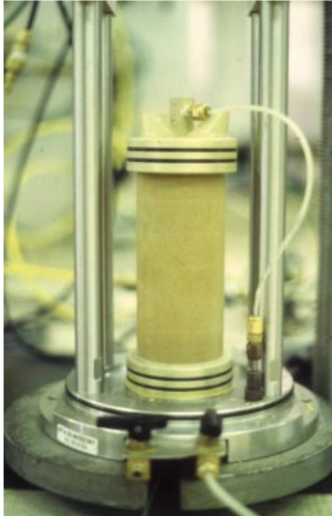
Figure 8.8 – Specimen with Internal Vacuum Applied
