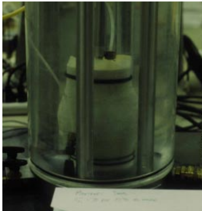
Figure 8.12 - Specimen Condition After Bulging Failure
