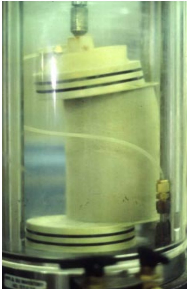
Figure 8.4 – Large Unidirectional Displacement of Specimen with Lubricated Ends
