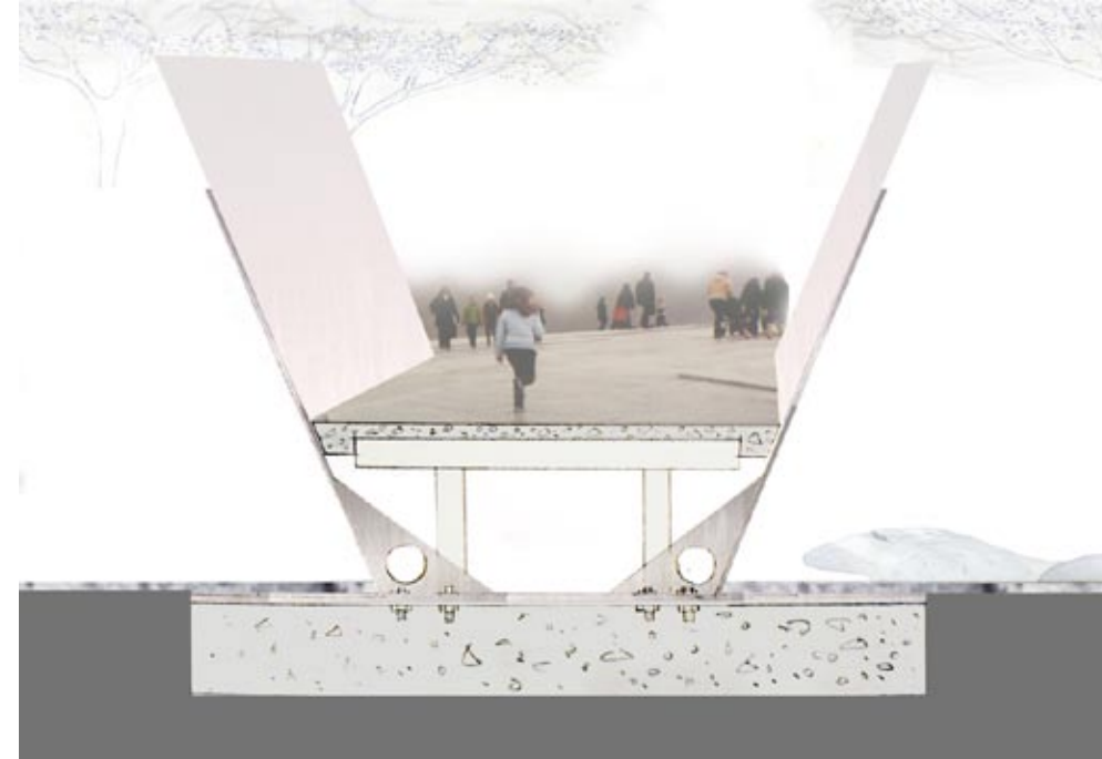
Figure 85. Detail Section of sunken plaza
