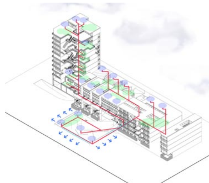
Figure 50. Rain water recycle system
