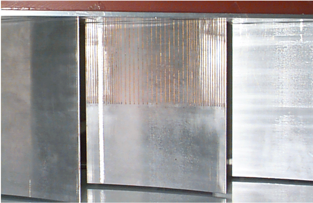
Figure 2-11: GE Rotor B blades mounted in the cascade tunnel; view shown from the trailing edge.
