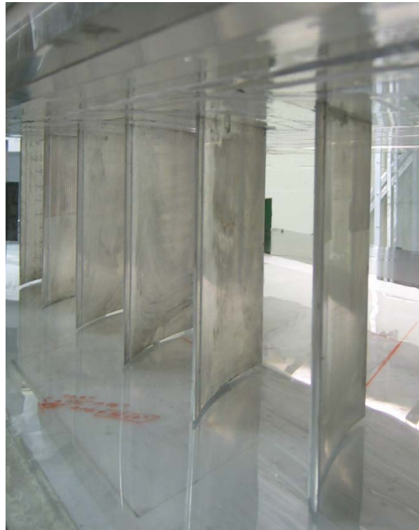
Figure 2-1: GE Rotor B blades mounted in Virginia Tech's linear cascade tunnel
