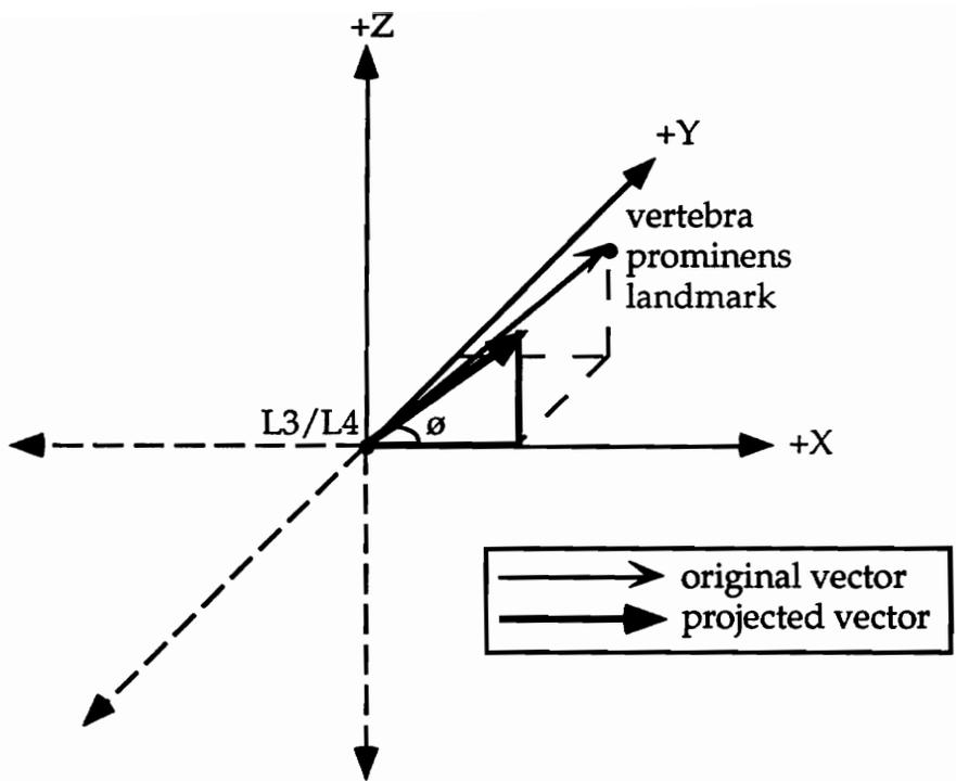
Figure 23. Torso lateral bending angle as projected upon the XZ (frontal) plane.
