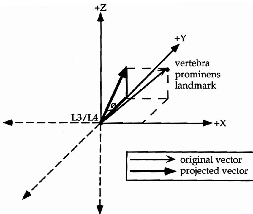
Figure 22. Torso extension/flexion angle as projected upon the YZ (sagittal) plane.
