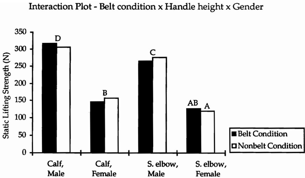
**Figure 29.** *Belt condition x Handle height x Gender* interaction plotted against upward lift force (N). (Conditions with same letters are not significantly different using a Newman-Keuls post hoc comparison test.)
