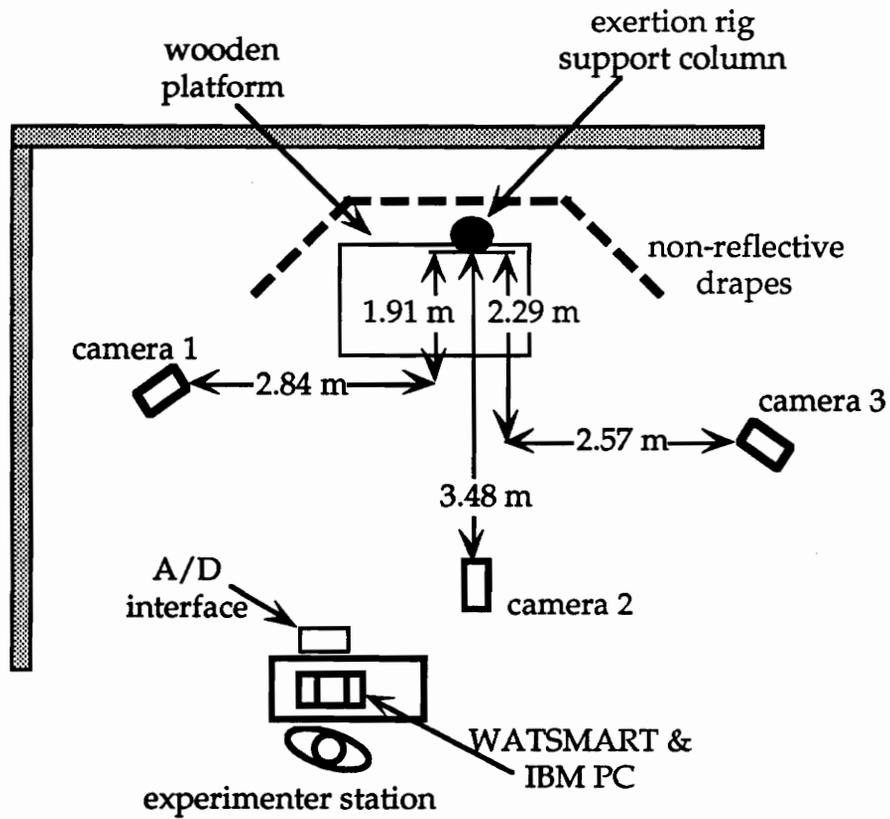
**Figure 7.** Layout of the experimental apparatus.
