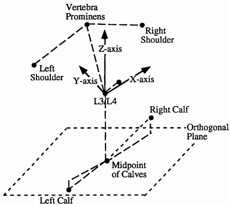
Figure 21. The axes of the body coordinate system as defined by the vectors  $\beta$ ,  $\delta$ , and  $\gamma_1$  (X, Y, and Z - axes, respectively).
