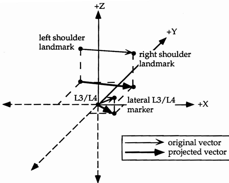
Figure 24. Axial twist angle as projected upon the XY (transverse) plane.
