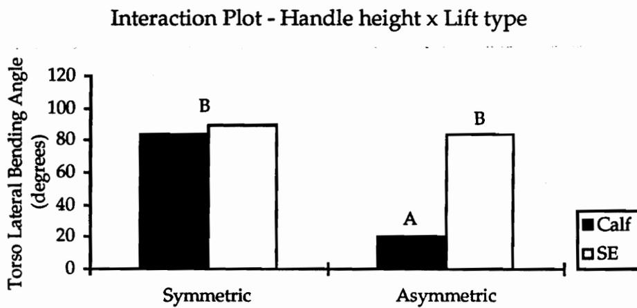
**Figure 26.** *Handle height x Lift type* interaction plotted against torso lateral bending angle. (Conditions with same letters are not significantly different using a Newman-Keuls post hoc comparison test.)
