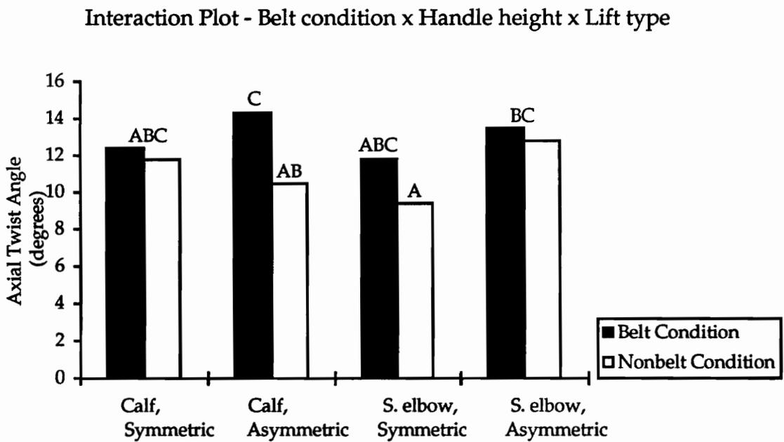
**Figure 27.** *Belt condition x Handle height x Lift type* interaction plotted against angle of axial twist of the shoulders. (Conditions with same letters are not significantly different using a Newman-Keuls post hoc comparison test.)
