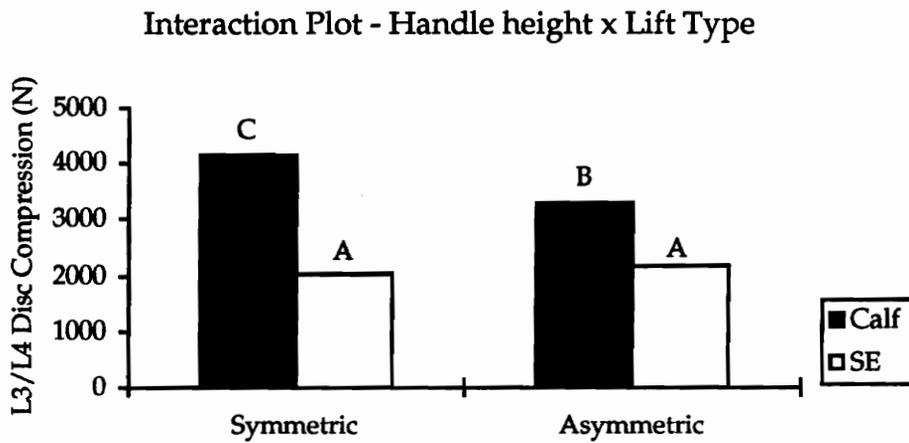
**Figure 31.** *Handle height x Lift type* interaction plotted against L3/L4 intervertebral disc spinal compression (N). (Conditions with same letters are not significantly different using a Newman-Keuls post hoc comparison test.)
