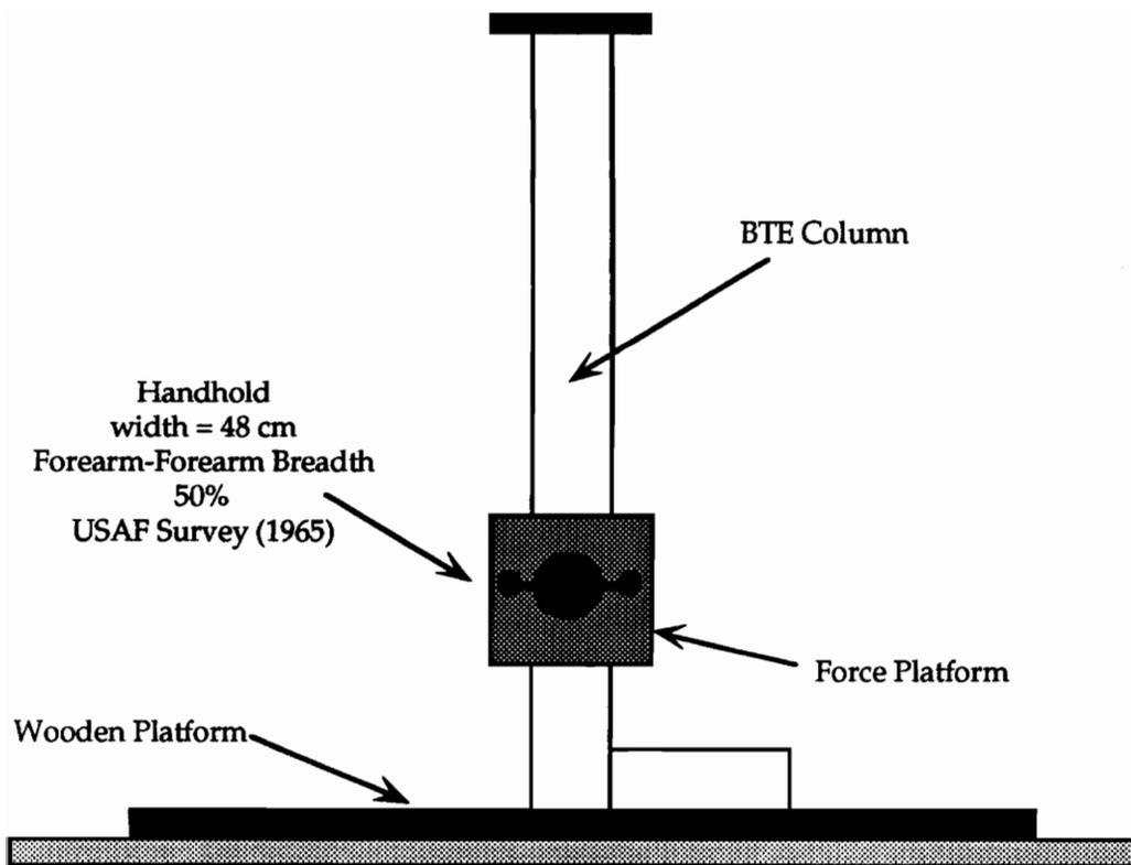
Figure 8. Schematic of the BTE rig.
