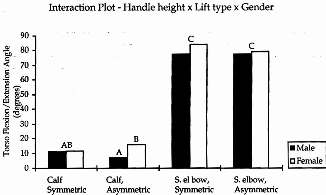
**Figure 25.** *Handle height x Lift type x Gender* interaction plotted against torso flexion/extension angle. (Conditions with same letters are not significantly different using a Newman-Keuls post hoc comparison test.)
