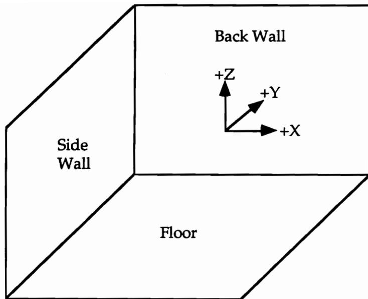
**Figure 20.** Orientation of the room coordinate system.
