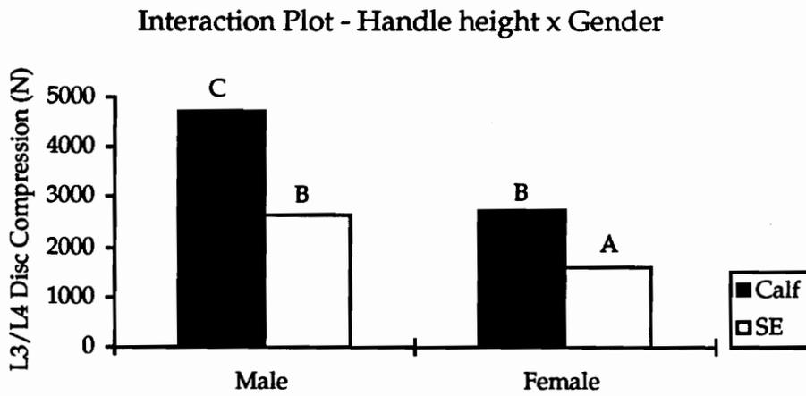
**Figure 30.** *Handle height x Gender* interaction plotted against L3/L4 intervertebral disc spinal compression (N). (Conditions with same letters are not significantly different using a Newman-Keuls post hoc comparison test.)
