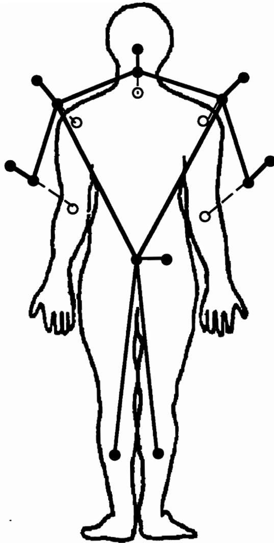
**Figure 11.** Posterior view of WATSMART IRED diode placement.
