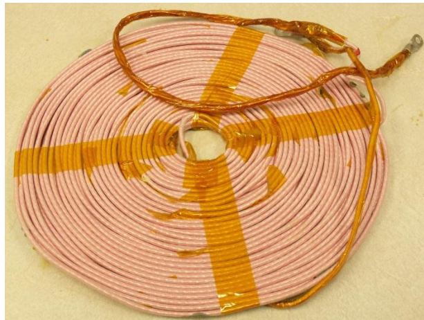
Figure 2.8 Induction Coil with 60 turns and 473uH inductance
