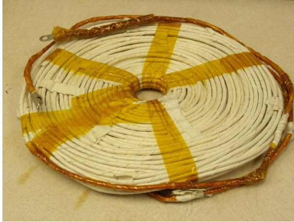
Figure 2.9 Induction Coil with 96 turns and 1.126mH inductance
