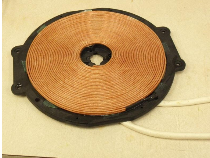
Figure 2.7 Induction Coil with 32 turns and 147uH inductance
