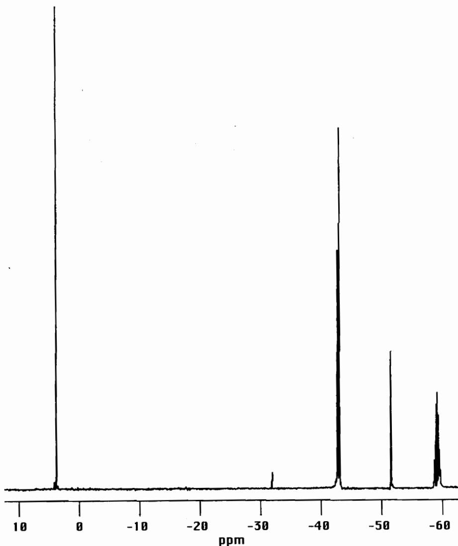
Figure 2.4: 200 MHz ^{31}\text{P} NMR Spectrum of [\text{Ir}(\text{D})(1,5\text{-COD})(\text{PMe}_3)_3](\text{Cl})(\text{O}_2\text{P}(\text{OCH}_2\text{Ph})_2)
