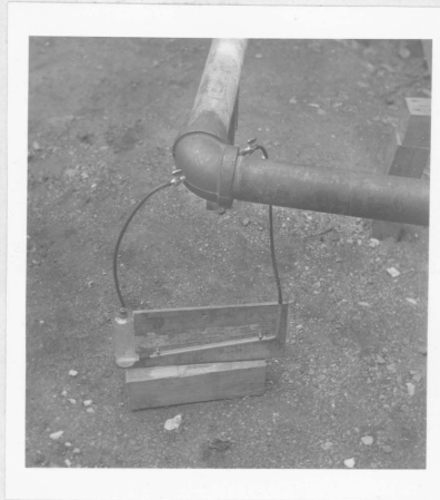
Fig. 7. Three-inch Elbow Flow Meter and Manometer
