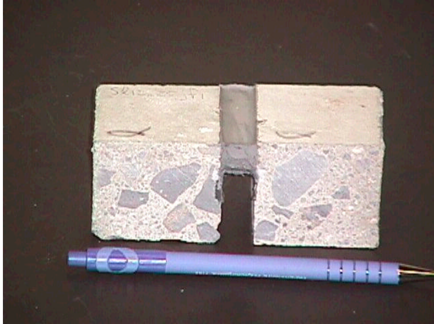
Figure D.3 Top of specimen SL12_25JF1 after environmental conditioning and cyclic loading
