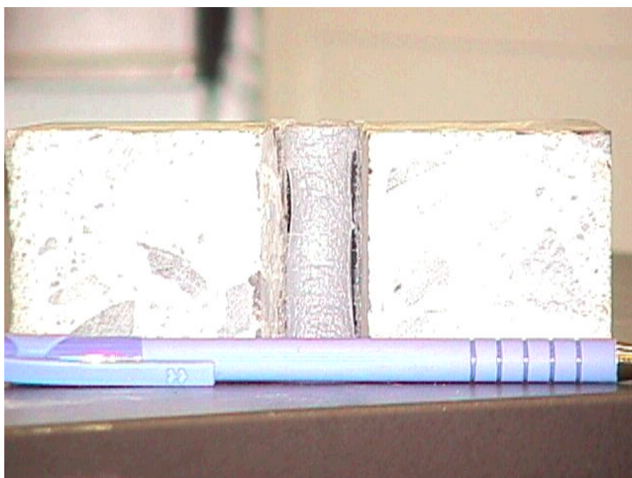
Figure D.18 Bottom of specimen SL12_25_1 after environmental conditioning and cyclic loading
