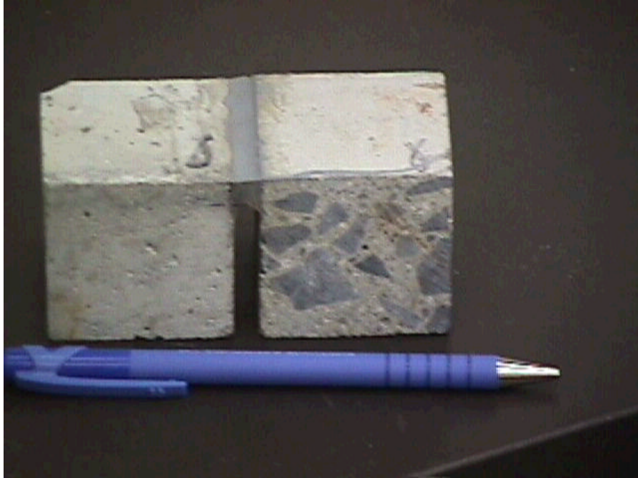
Figure D.5 Top of specimen SL6_25JF2 after environmental conditioning and cyclic loading
