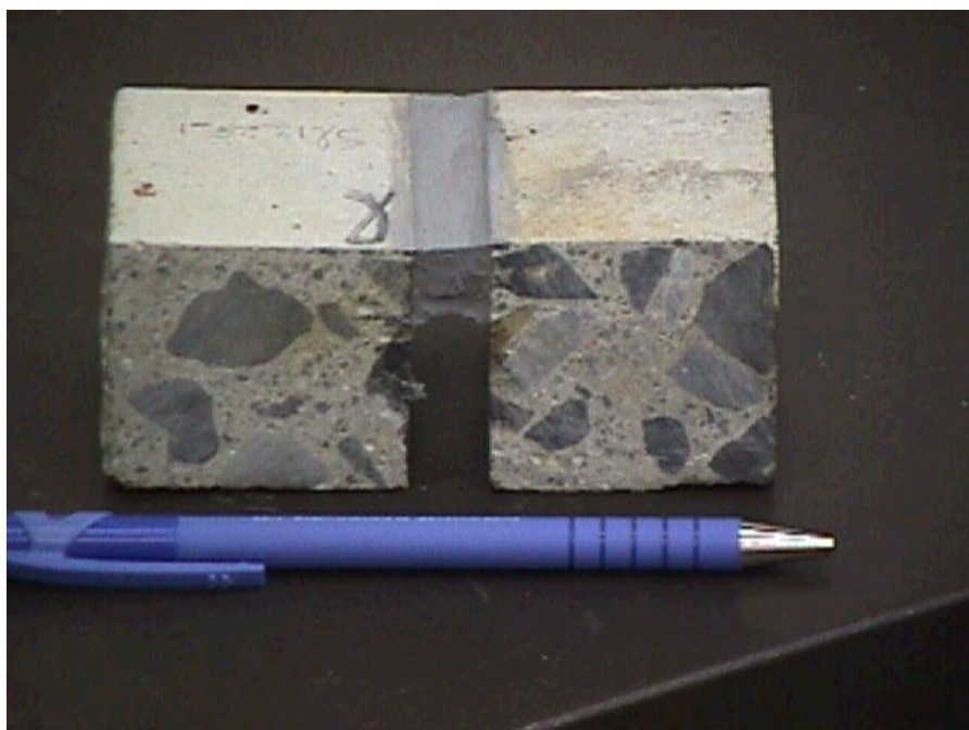
Figure D.17 Top of specimen SL12_25_1 after environmental conditioning and cyclic loading
