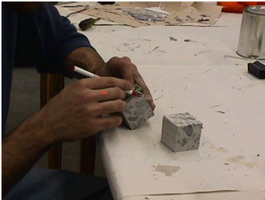
Figure A.16 Marking the sealant depth on the concrete cubes
