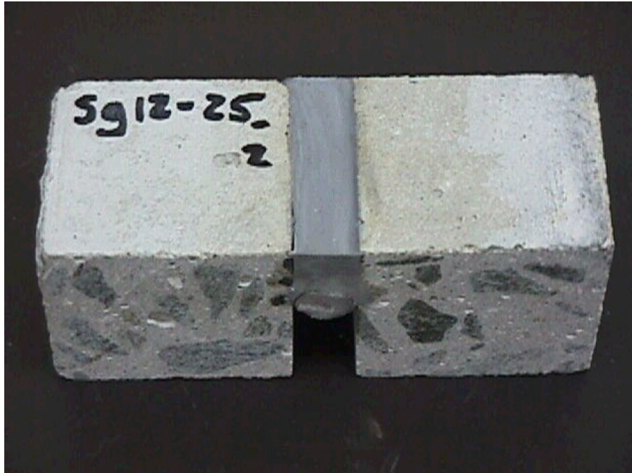
Figure D.13 Top of specimen SG12_25_2 after environmental conditioning and cyclic loading
