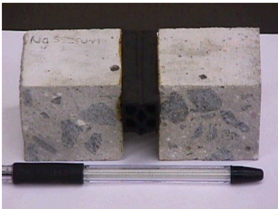
Figure D.29 Top of specimen NGS25UV1 after environmental conditioning and cyclic loading
