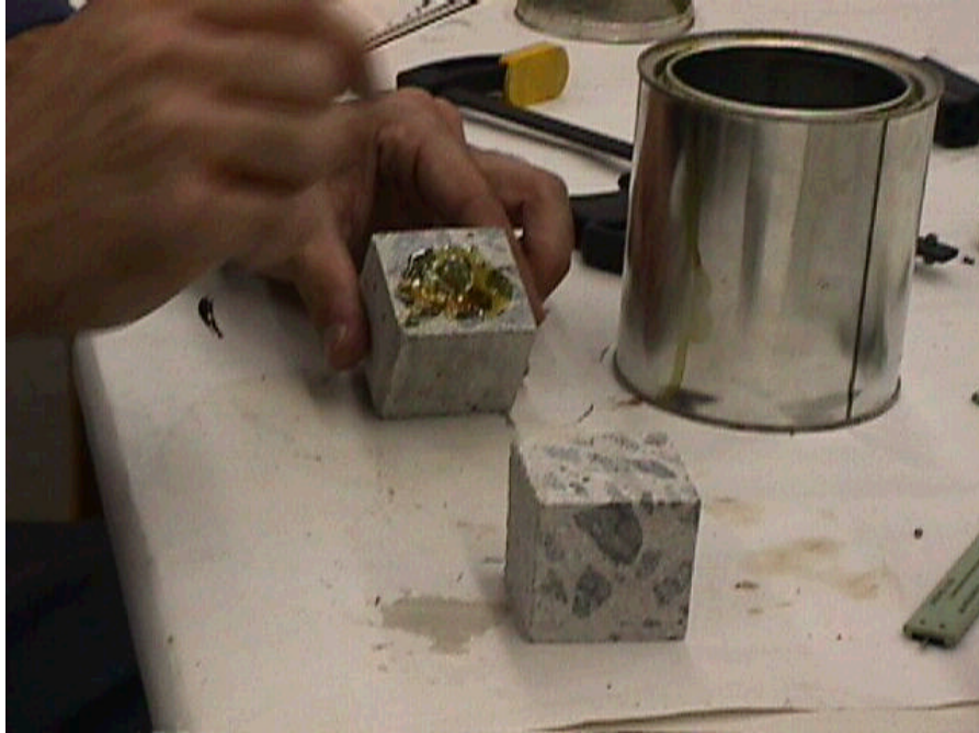
Figure A.17 Applying the lubricant/adhesive to the concrete joint wall
