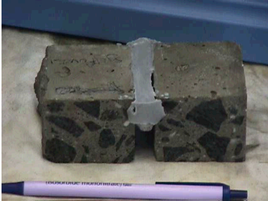
Figure B.5 Silicone specimen with 6.35 mm joint width after 1000 hours of exposure to UV and two days of exposure to jet fuel
