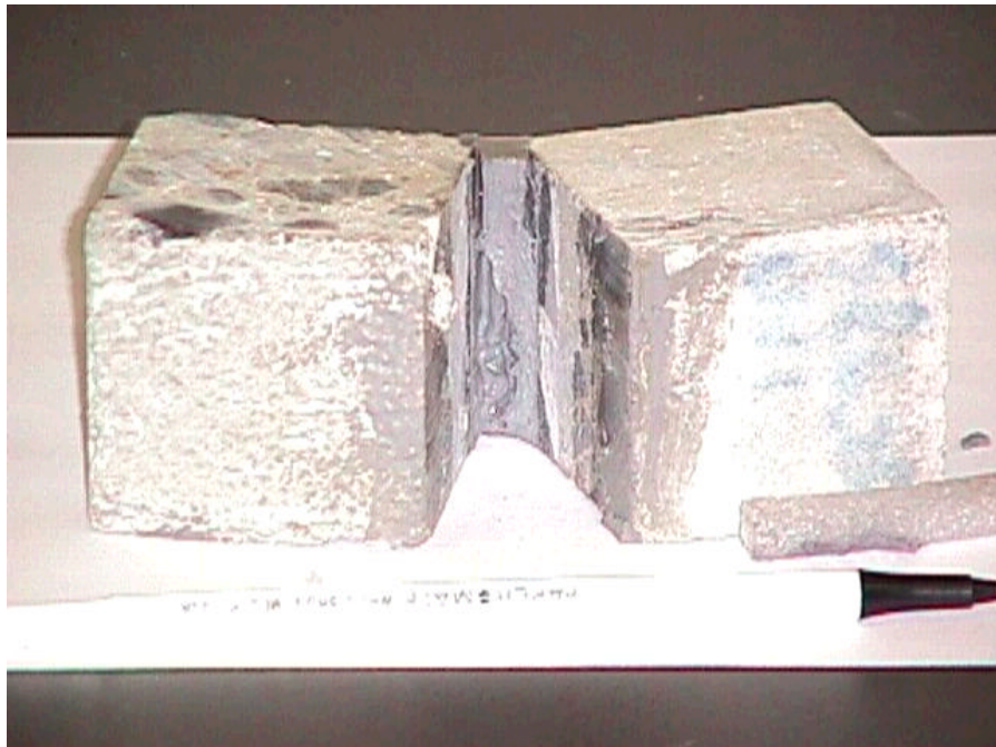
Figure D.12 Bottom of specimen SL6_25UV1 after environmental conditioning and cyclic loading
