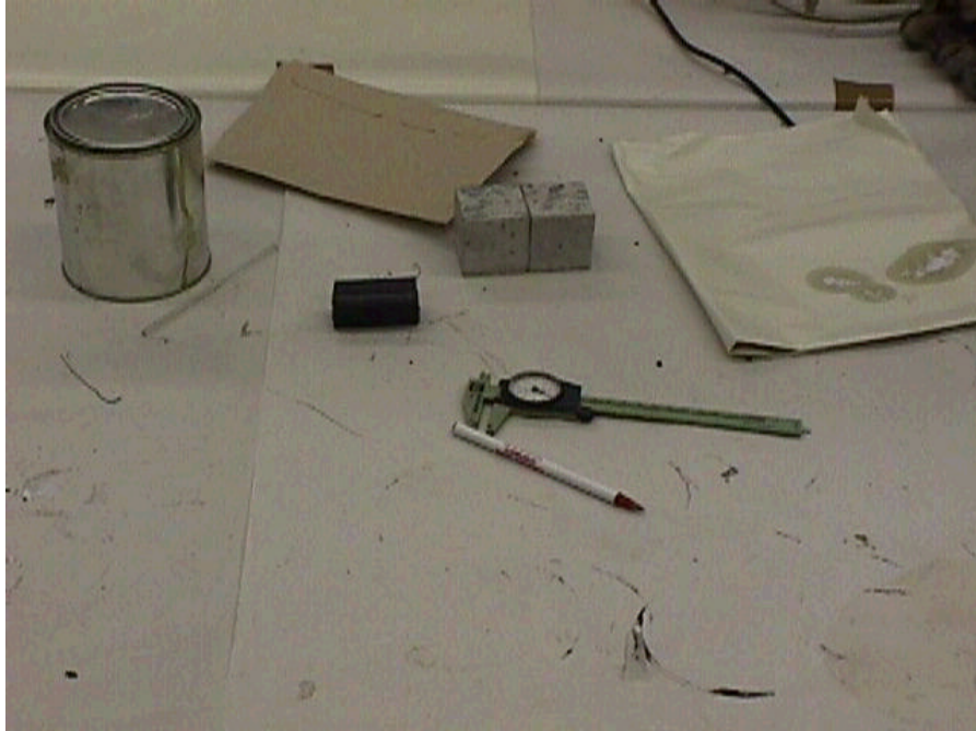
Figure A.15 Tools and components needed to fabricate neoprene test specimens
