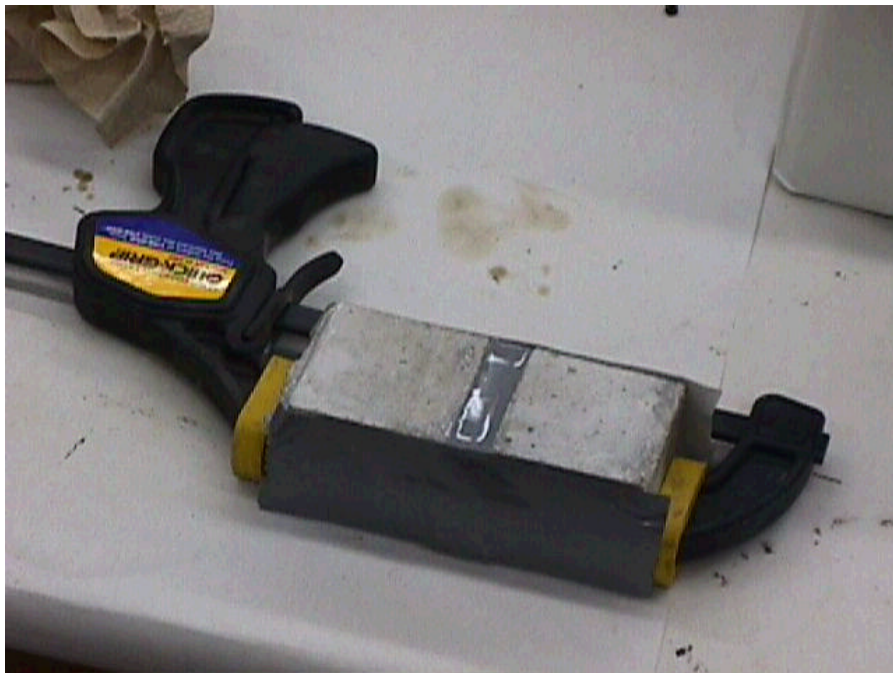
Figure A.14 The sealant is allowed to cure for 21 days
