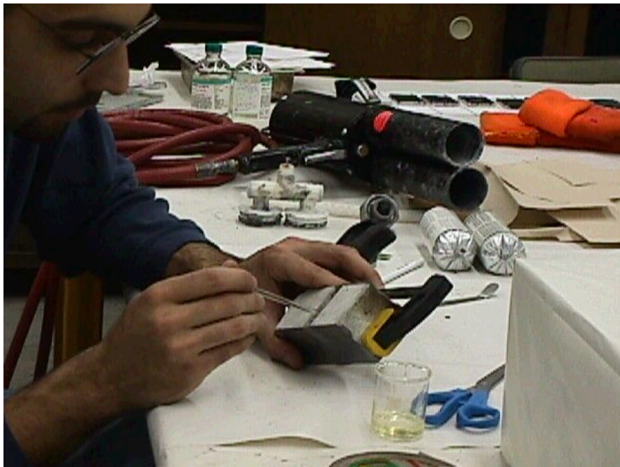
Figure A.8 Applying the primer to the concrete joint wall
