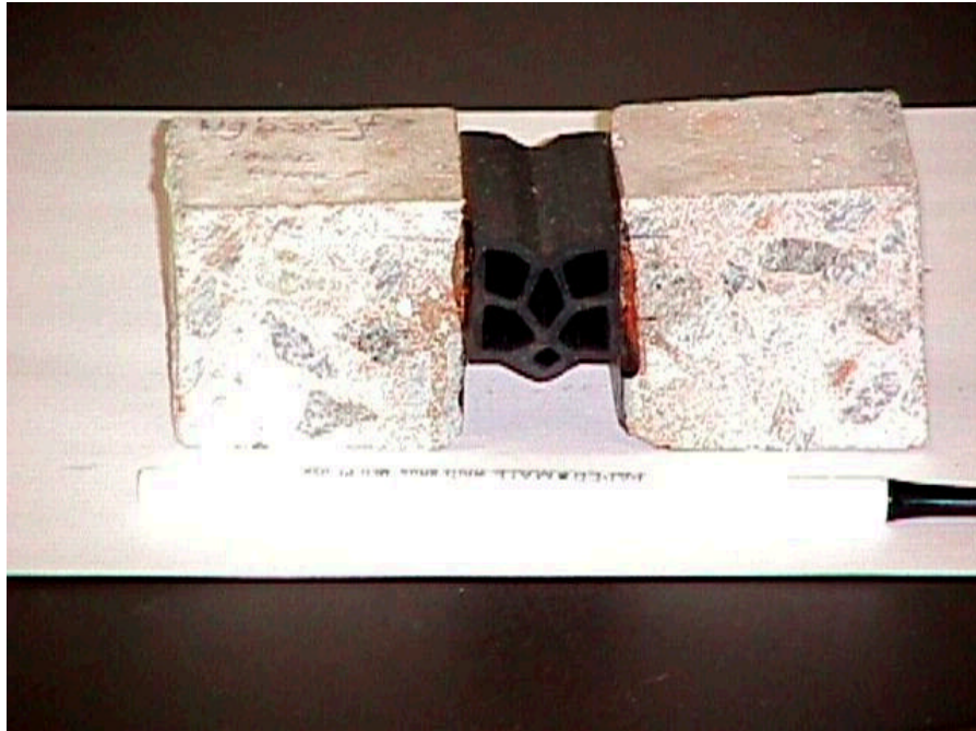
Figure D.21 Top of specimen NGB25JF2 after environmental conditioning and cyclic loading
