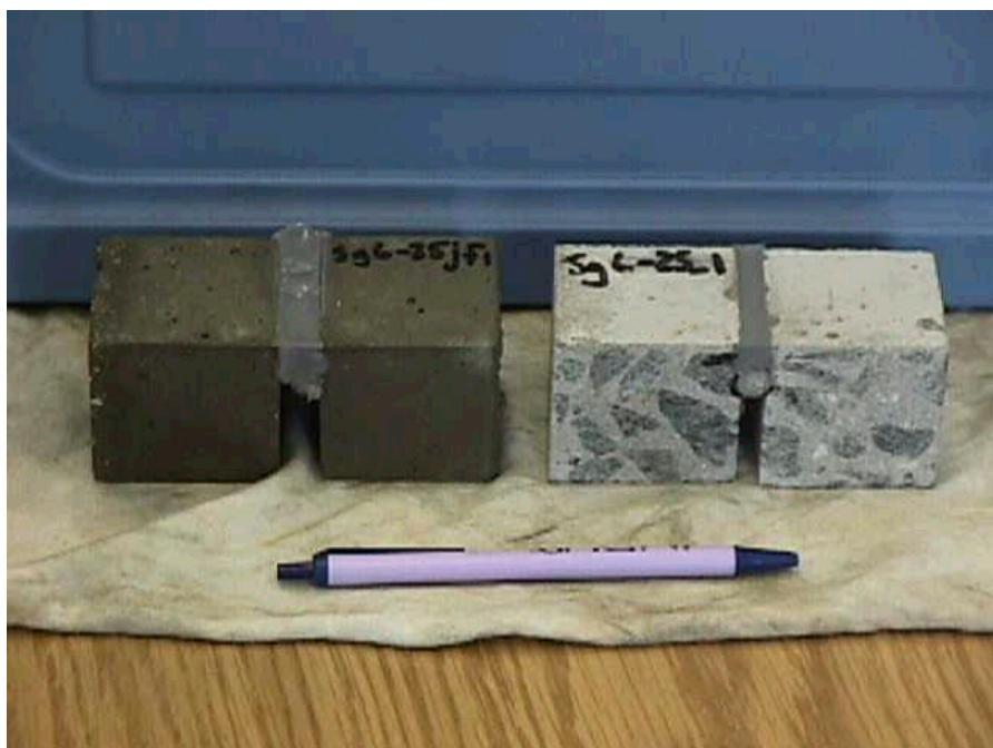
Figure B.1 Silicone specimen with 6.35 mm joint width after two days of exposure to jet fuel
