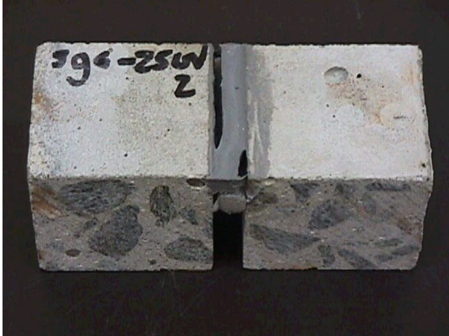
Figure D.7 Top of specimen SG6_25UV2 after environmental conditioning and cyclic loading
