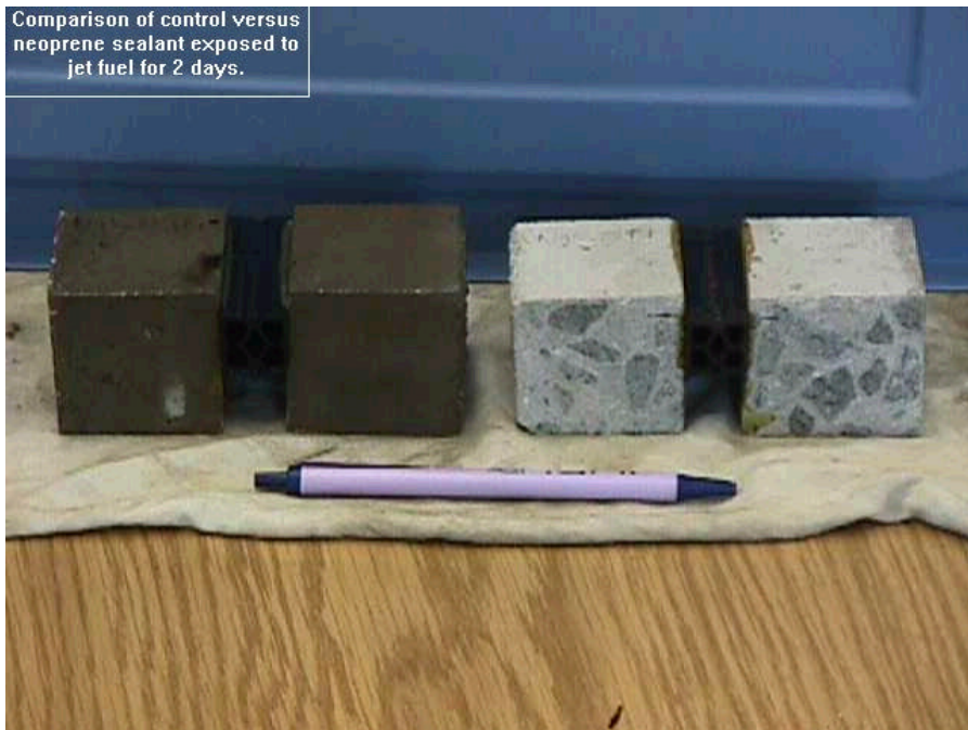
Figure B.6 Small neoprene specimen after two days of exposure to jet fuel
