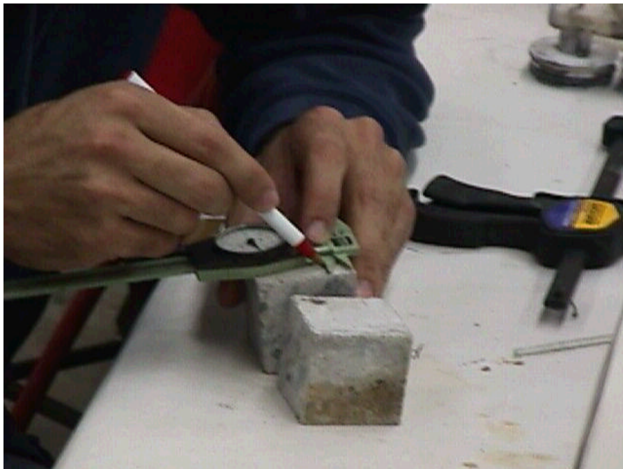
Figure A.2 Marking the sealant depth on the concrete cubes
