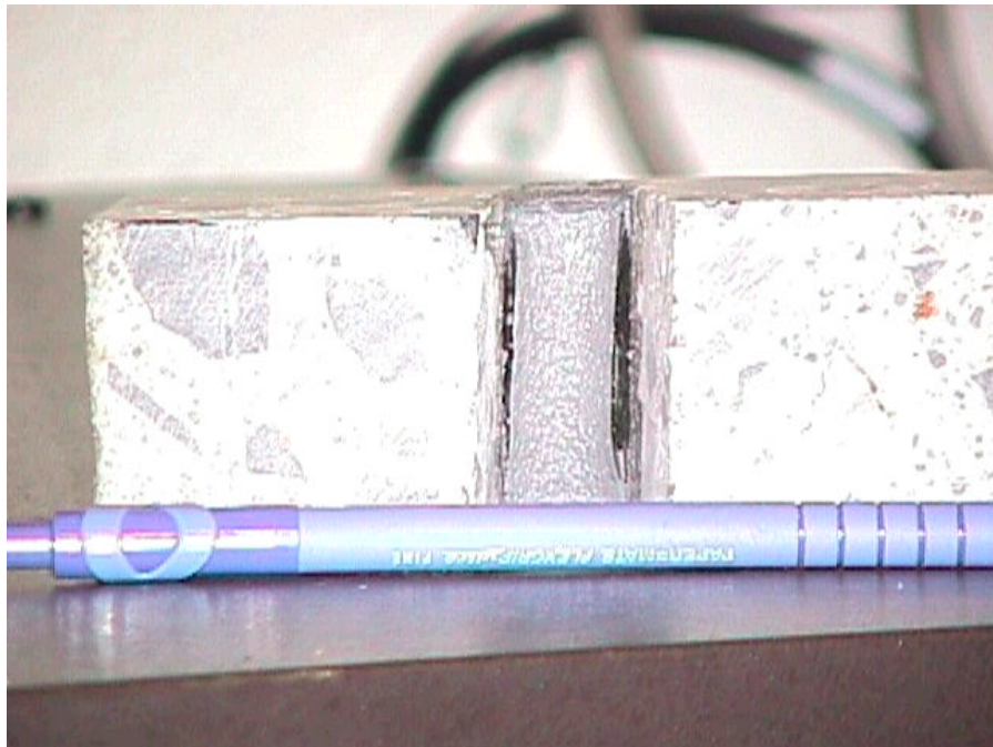
Figure D.4 Bottom of specimen SL12_25JF1 after environmental conditioning and cyclic loading
