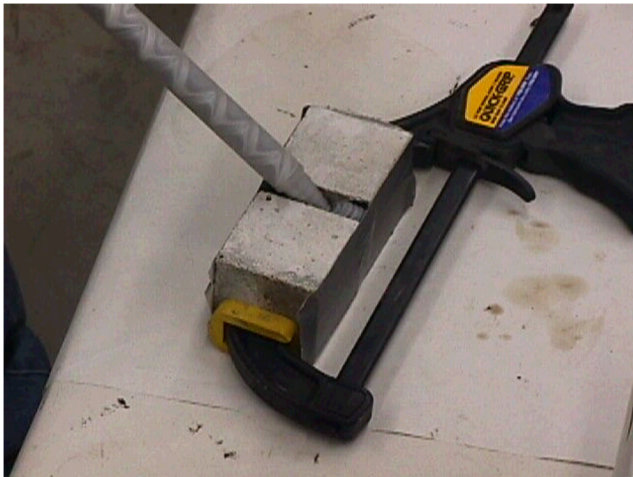
Figure A.12 Sealant injection into the joint
