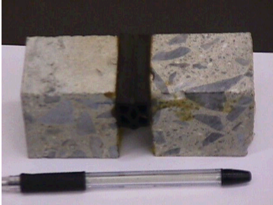
Figure D.31 Top of specimen NLS25UV1 after environmental conditioning and cyclic loading
