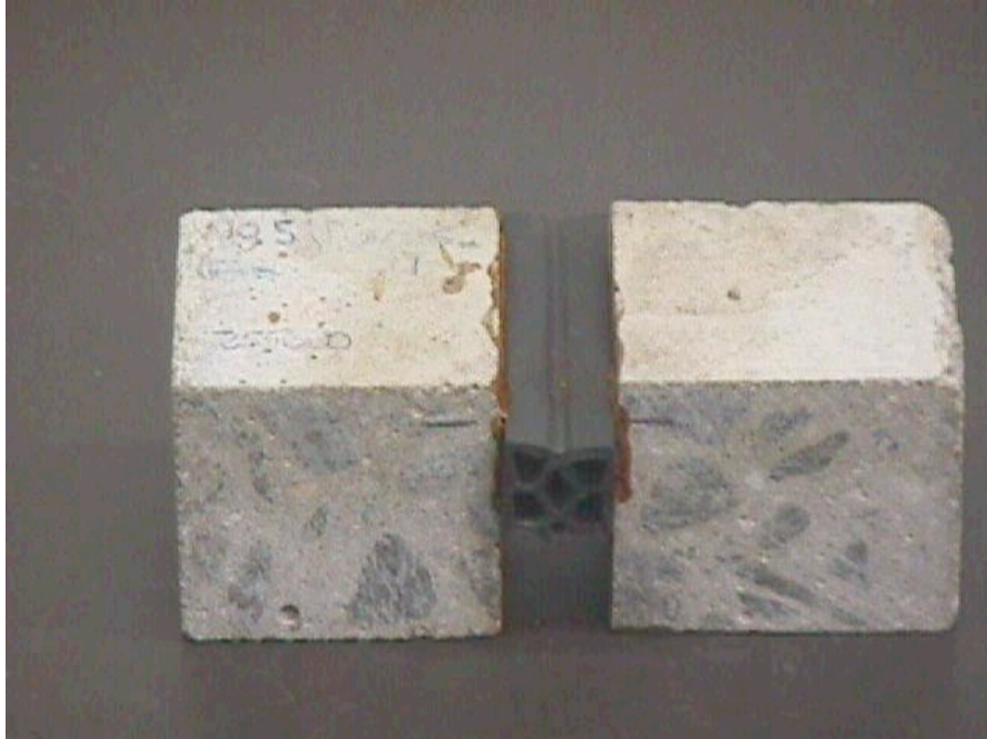
Figure D.25 Top of specimen NGS25UVJF1 after environmental conditioning and cyclic loading
