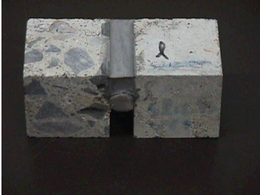
Figure D.9 Top of specimen SL12_25UV1 after environmental conditioning and cyclic loading
