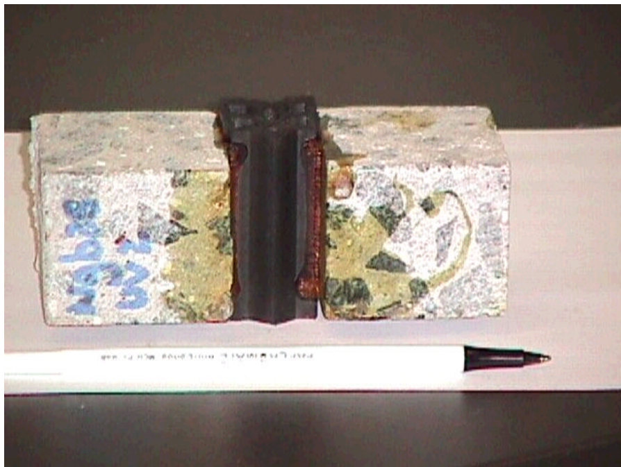
Figure D.24 Bottom of specimen NGB25UV2 after environmental conditioning and cyclic loading
