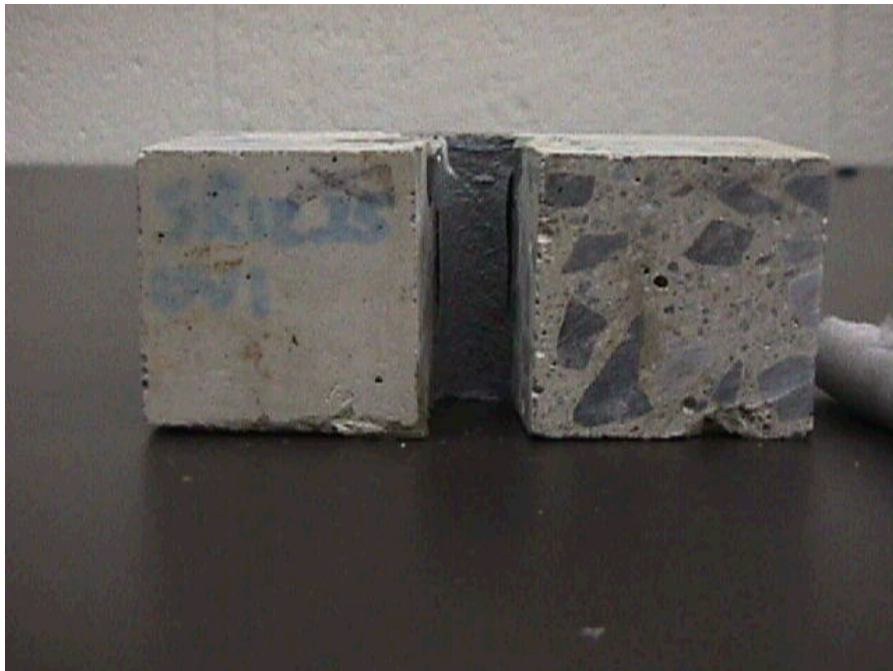
Figure D.10 Bottom of specimen SL12_25UV1 after environmental conditioning and cyclic loading
