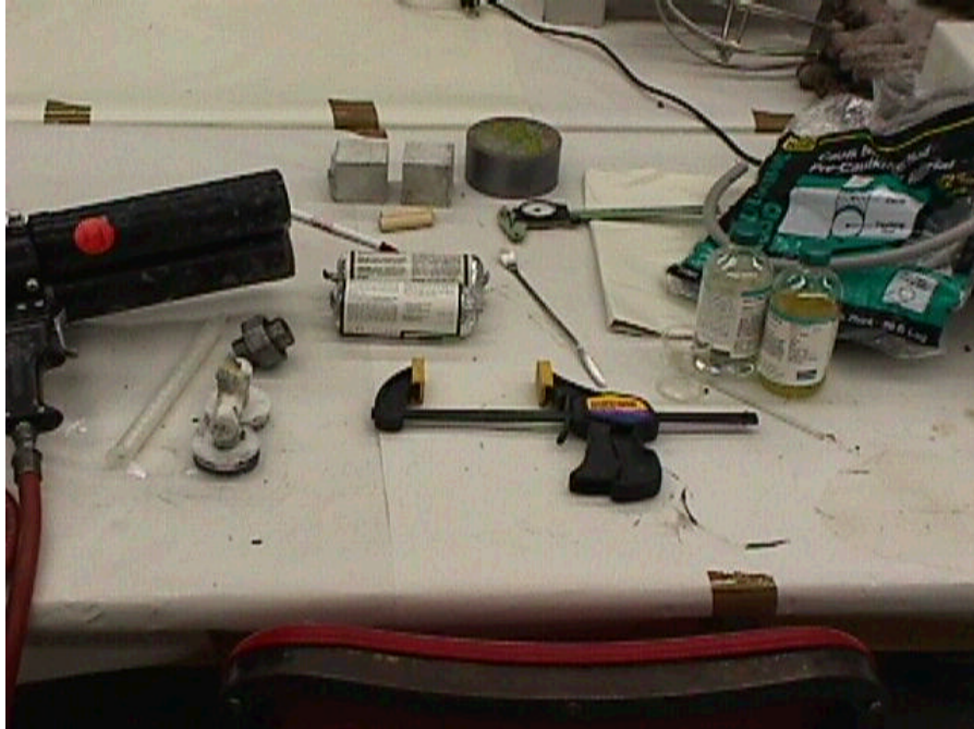
Figure A.1 Tools and components needed to fabricate silicone test specimens
