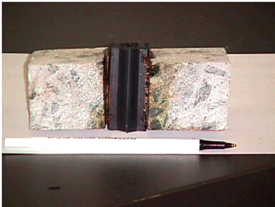
Figure D.22 Bottom of specimen NGB25JF2 after environmental conditioning and cyclic loading
