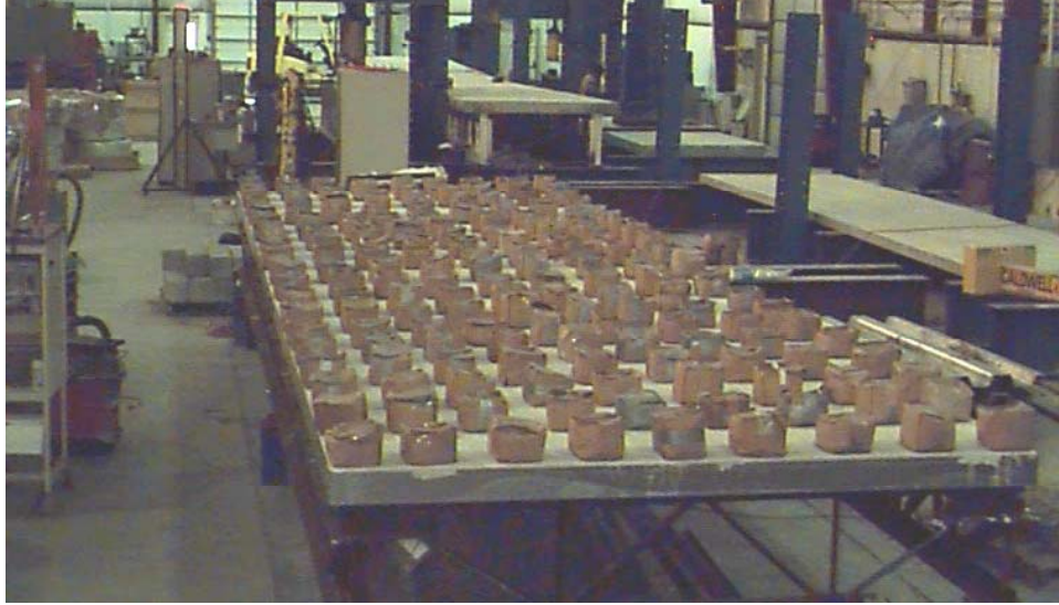
Figure 2. 6—Distributed Loading-15 psf
