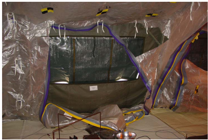
Figure 1.4: Post Blast figure for TEMPER Tent showing back side damage with tearing
