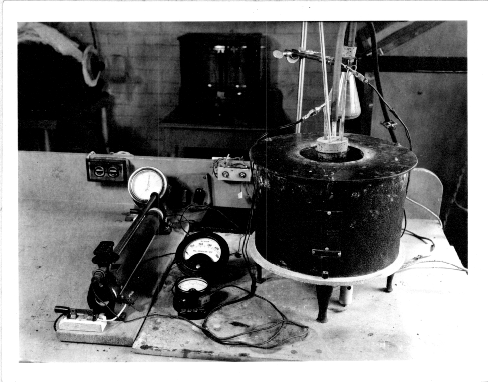
FIGURE 7. PHOTOGRAPH OF APPARATUS ARRANGED FOR ELECTROLYTIC STUDY OF ALUMINUM POLYSULFIDE AND POTASSIUM POLYSULFIDE SYSTEM
