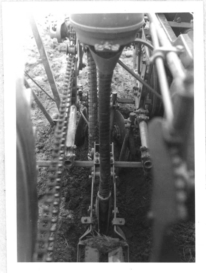
Fig. 13. A view of the same planting arrangement as shown in Fig. 11 operating in the field. Notice the position of the single disk hiller throwing clean soil into the path of the planter. This action resulted in more efficient coverage of the seed.
