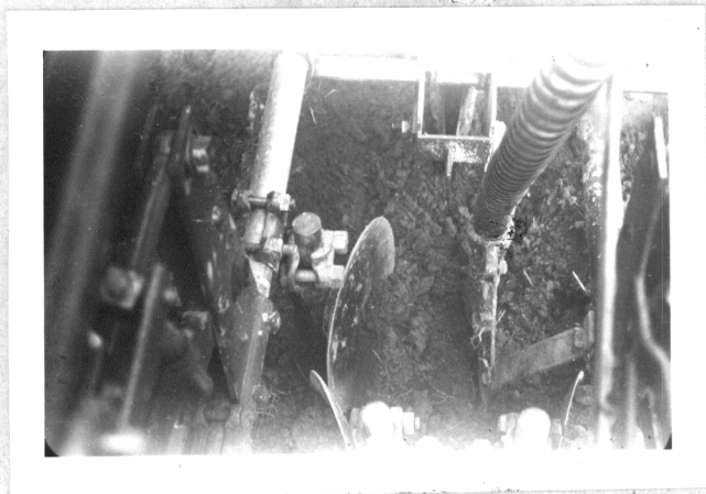
Fig. 15. A top view showing in detail the action of the single disk hiller in throwing clean soil into the path of the planter shoe. The double-disk furrow opener is seen following the single disk hiller and fertilizer shoe. The pair of disk hillers extend out of the bottom of the picture.
