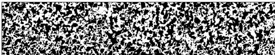
Figure 3.14. SOFC cathode active layer: threshold image (LSM only), two-point statistics; white indicates LSM and black pore and YSZ.
