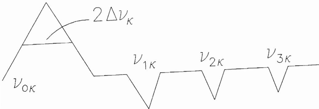
Figure 4: Resolved Stark shifts for a low J transition
