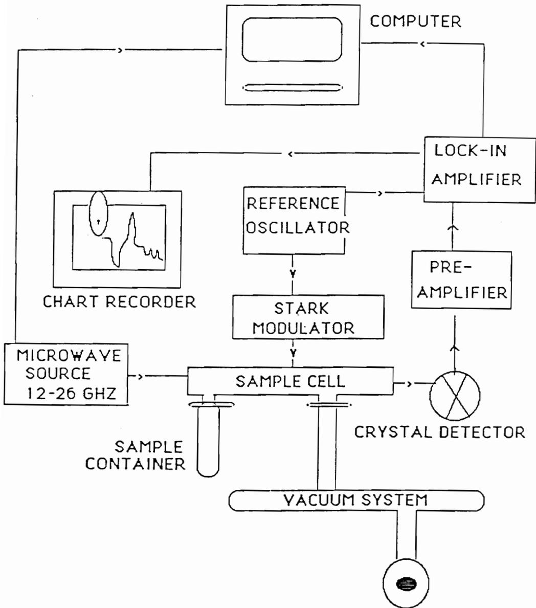
Figure 3: Schematic Diagram of the Stark Modulated Spectrometer
