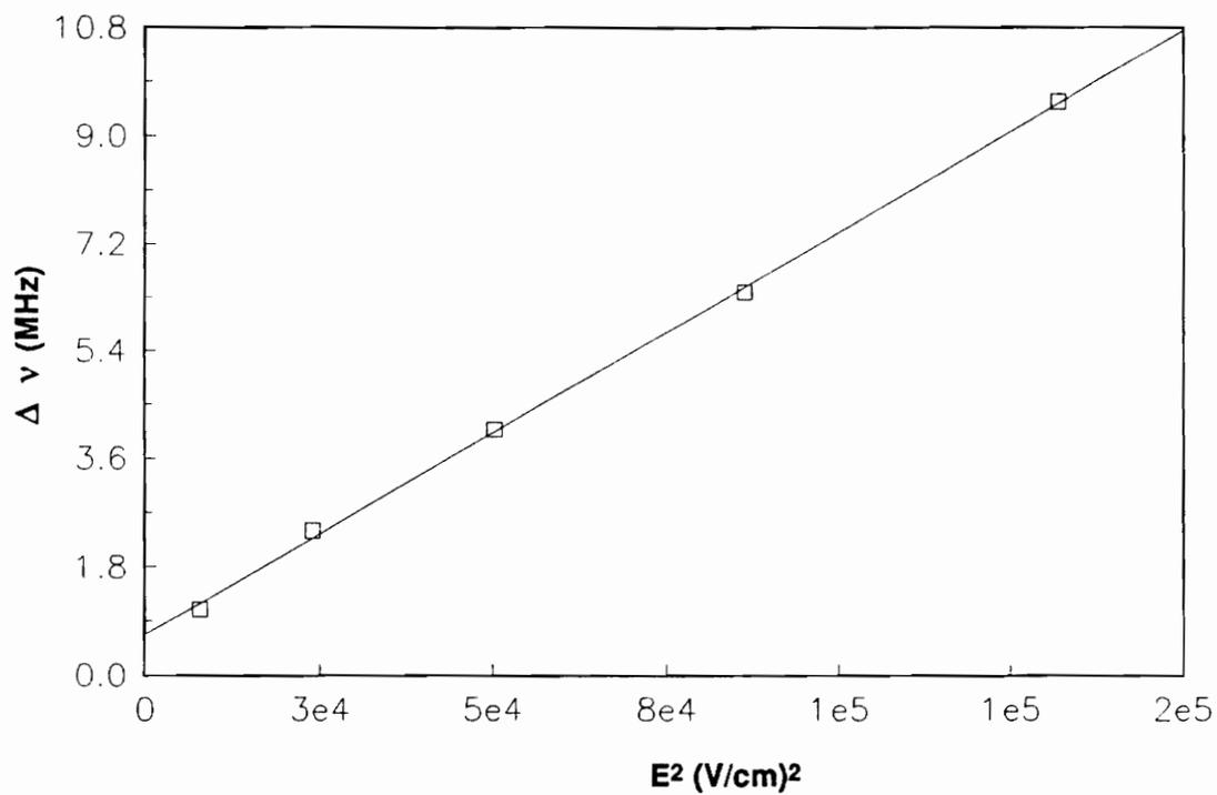
Figure 13:  $\Delta \nu$  vs  $\epsilon^2$  for the transition at 14049 MHz
