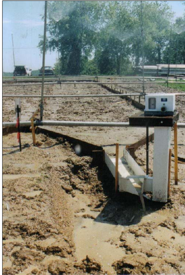
Figure 3.3 Rectangular flume attached to a stage recorder
