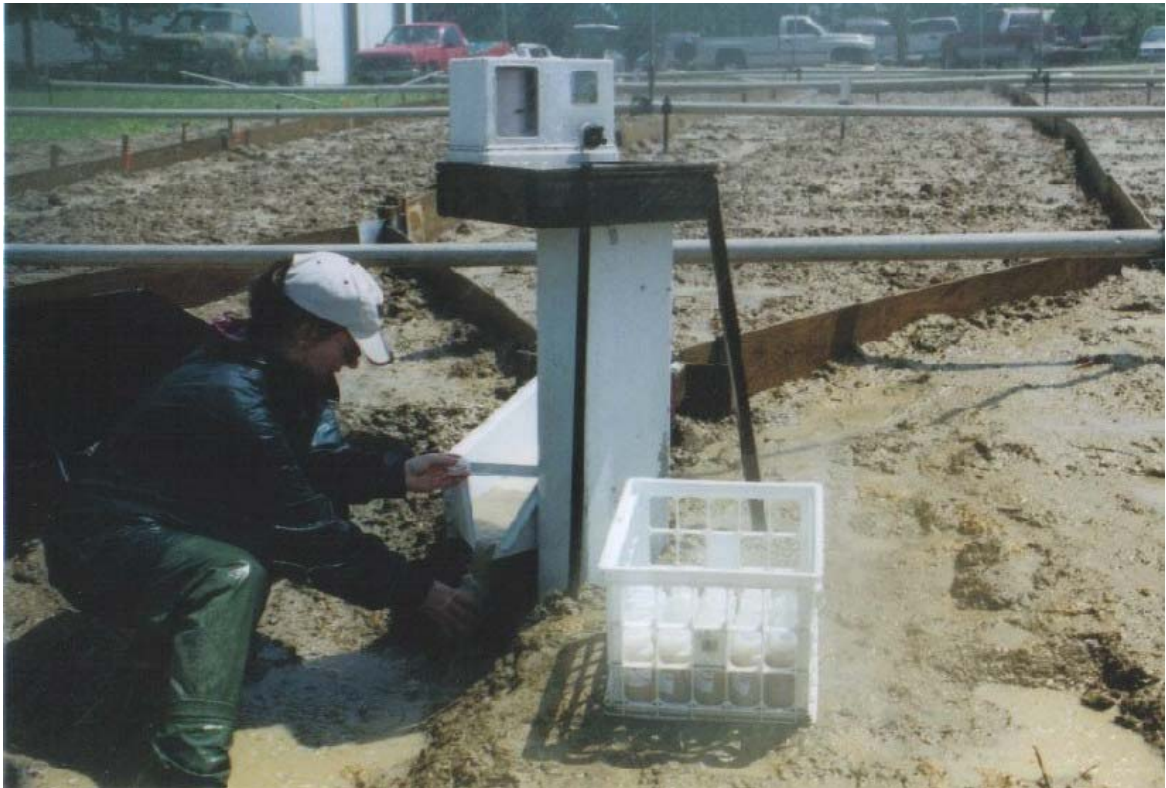
Figure 3.6 A graduate student (Tess Wynn) collecting samples of runoff flowing through the flume
