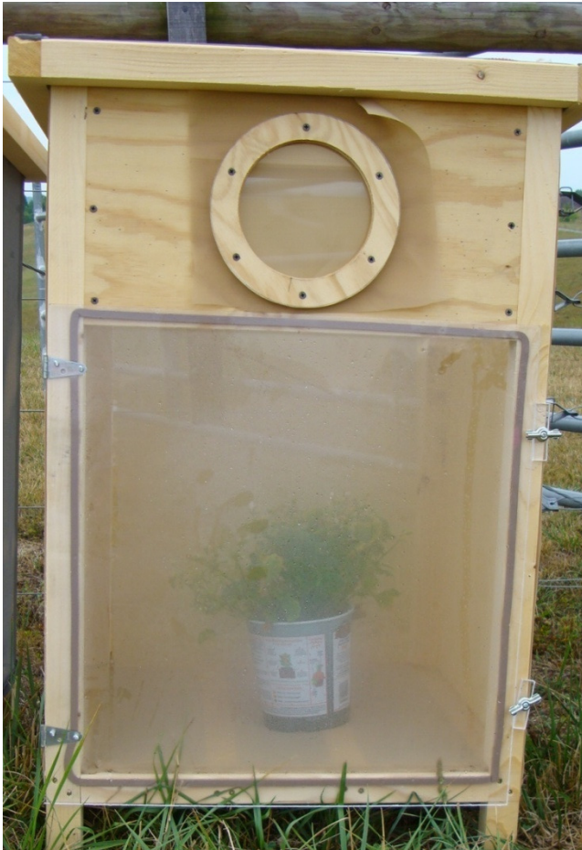
Figure 4.1 Nylon mesh, wood, and Plexiglas® cage designed to hold potted plants and Japanese beetles.
