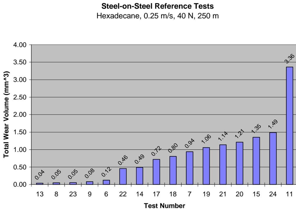
**Figure 4.1.1.1** Hexadecane Reference Tests in Order by Total Wear, Steel System.
