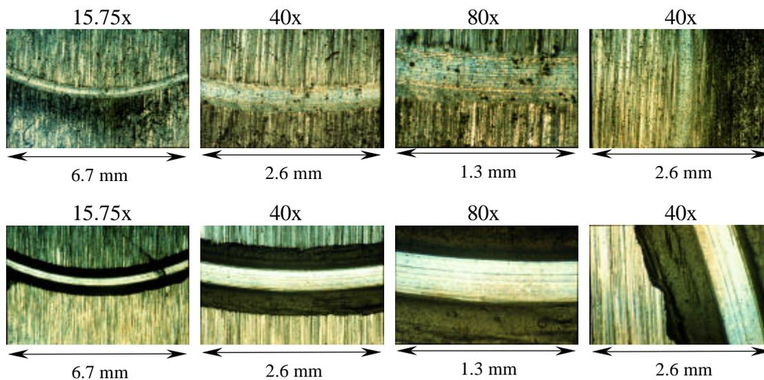
**Figure 4.1.2.8** Photomicrographs of Ethyl-4-Amino Benzoate Disk Wear Tracks in Steel System.
