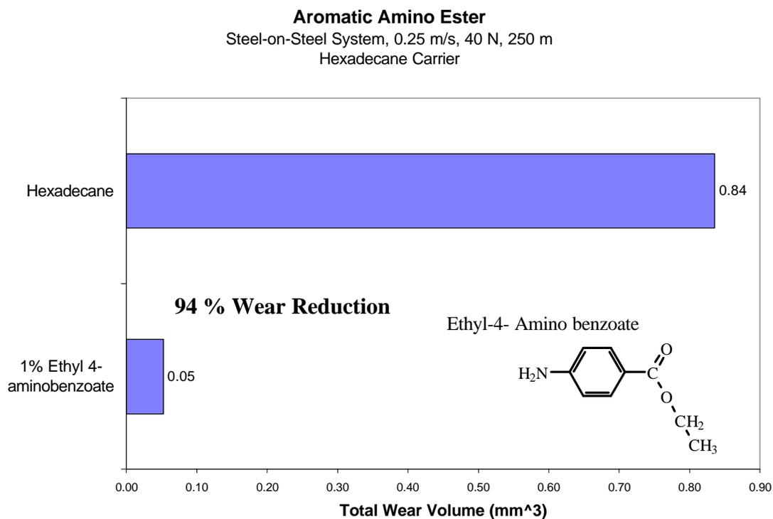
**Figure 4.1.2.7** Anti-wear Effect of Aromatic Amino Ester in Steel System.
