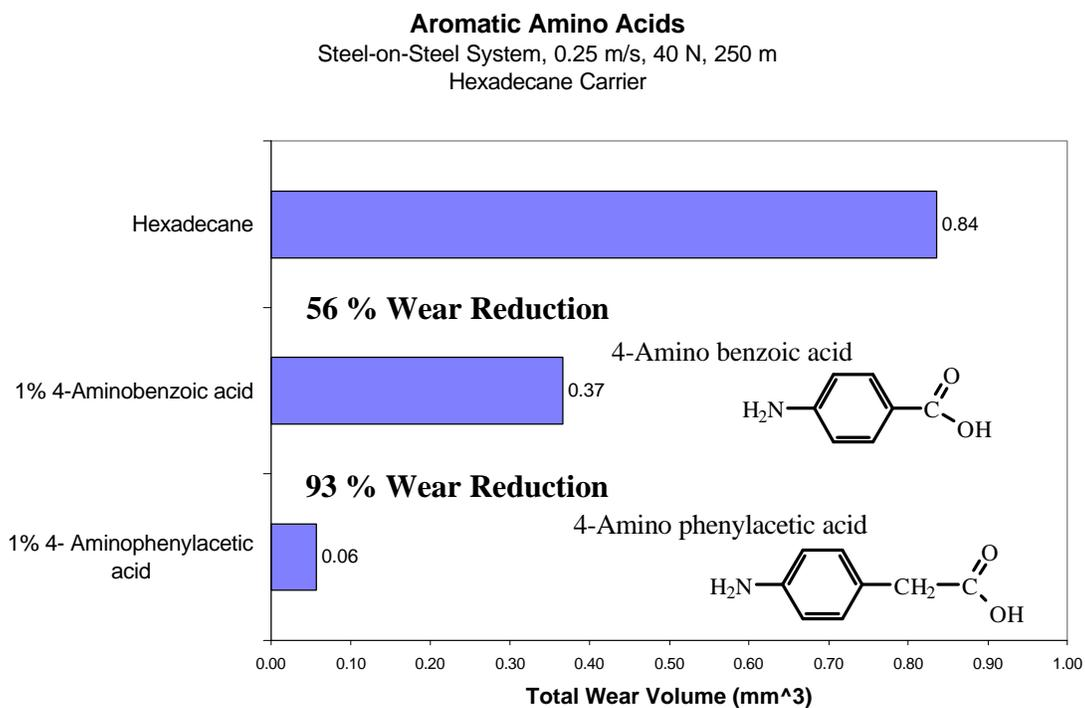
**Figure 4.1.2.4** Anti-wear Effects of Aromatic Amino Acids in Steel System.
