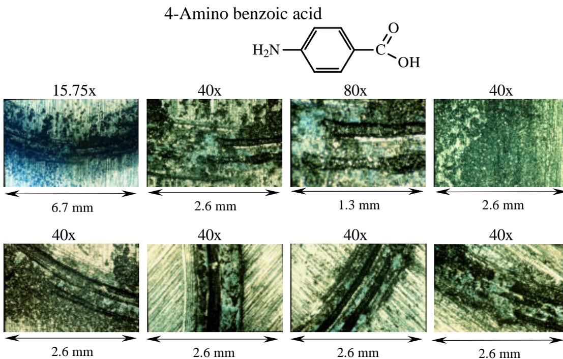
**Figure 4.1.2.5** Photomicrographs of 4-Amino Benzoic Acid Disk Wear Track in Steel System.
