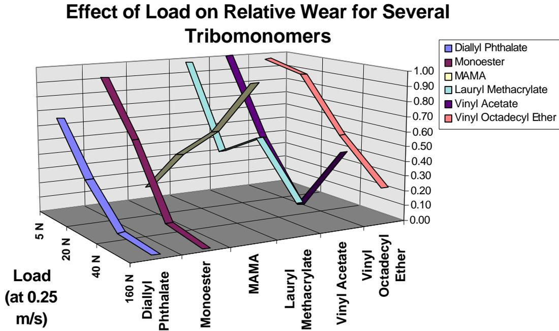
**Figure 2.5.1** Effect of Load on Relative Wear for Several Tribomonomers
