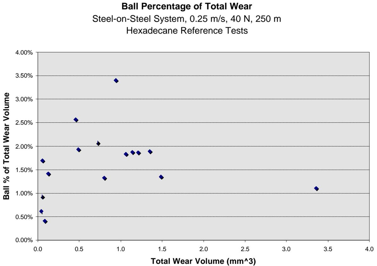
**Figure 4.1.1.2** Ball Percentage of Total Wear Volume for Hexadecane Reference Tests in Steel System.
