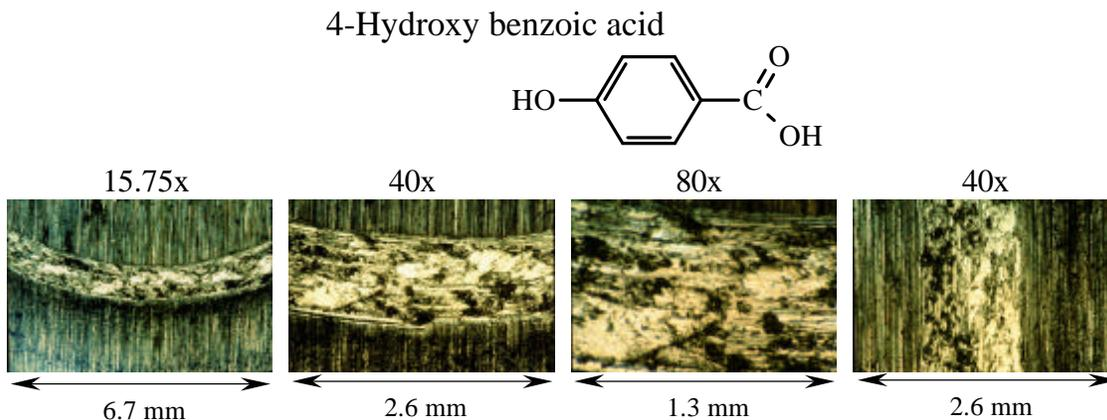
**Figure 4.1.2.2** Photomicrographs of 4-Hydroxy Benzoic Acid Disk Wear Track in Steel System (after methanol rinse).
