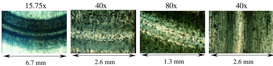
**Figure 4.1.3.2** Photomicrographs of Equimolar Mixture of Compounds Dimethyl Terephthalate and Tert-Butyl Hydroquinone Disk Wear Track in Steel System.
