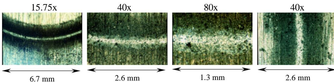
**Figure 4.1.2.6** Photomicrographs of 4-Amino Phenylacetic Acid Disk Wear Track in Steel System.
