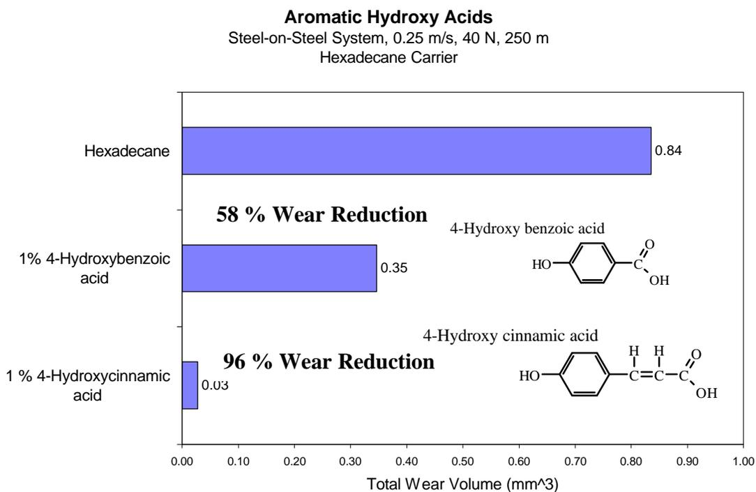
**Figure 4.1.2.1** Anti-wear Effects of Hydroxy Acids in Steel System.
