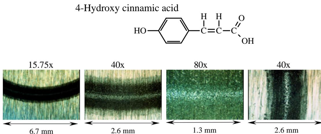
**Figure 4.1.2.3** Photomicrographs of 4-Hydroxy cinnamic acid Disk Wear Track in Steel System (after methanol rinse).
