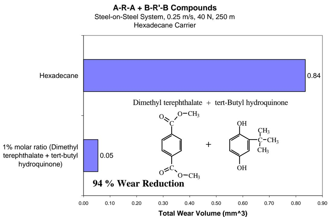
**Figure 4.1.3.1** Anti-wear Effect of A-R-A + B-R'-B Compounds Dimethyl Terephthalate and Tert-Butyl Hydroquinone in Steel System.
