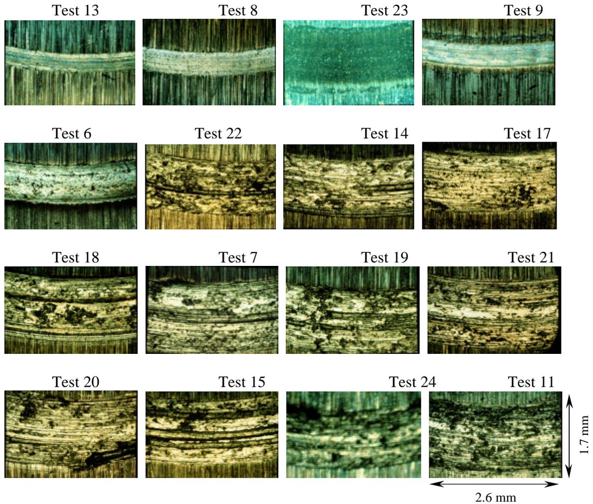
**Figure 4.1.1.3** Photomicrographs of Disk Wear Tracks for Hexadecane Reference Tests at 40x (All rinsed except Test 23)
