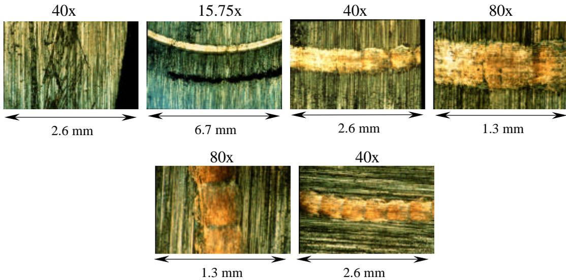
**Figure 4.1.4.2** Photomicrographs of Caprolactam Disk Wear Track in Steel System.
