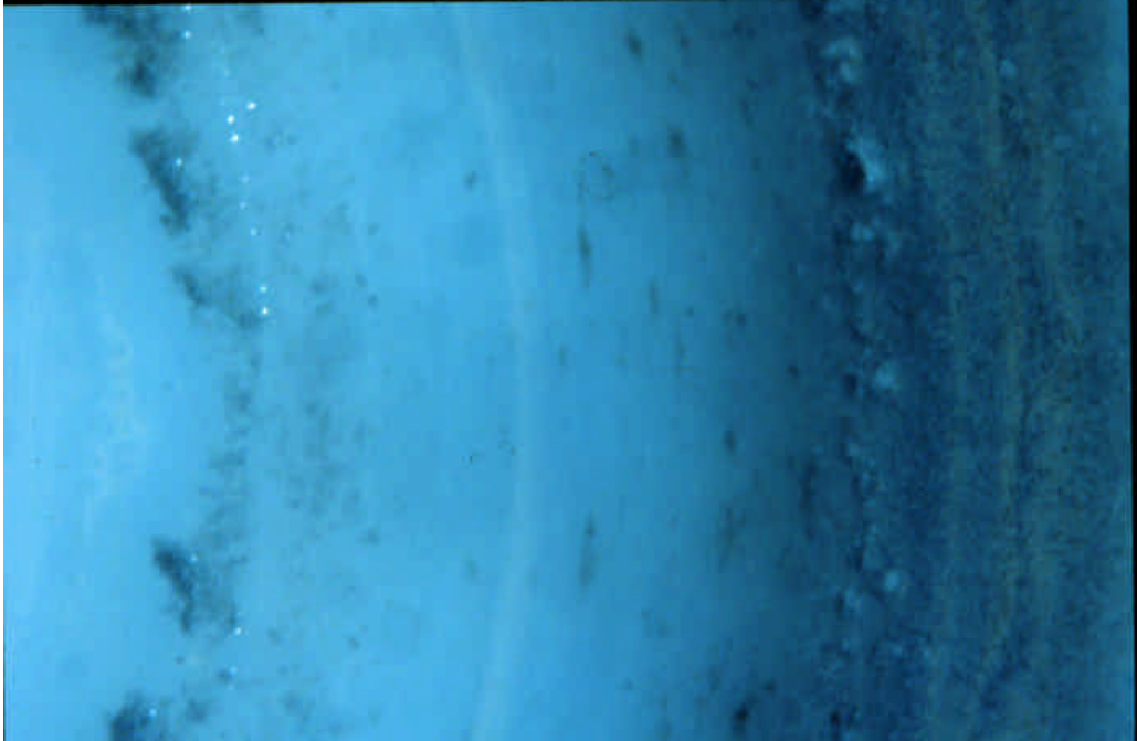
Figure 4.2.1.5 Alumina A System Reference, Test 29: Photomicrograph of Disk Wear Track (15.75 x)
