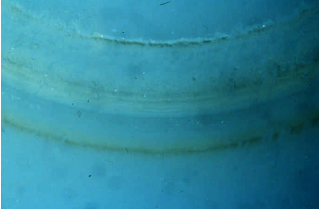
Figure 4.2.3.3 Dimethyl Terephthalate and Tert-Butyl Hydroquinone in Alumina A System, Test 38: Photomicrograph of Disk Wear Track (15.75 x)
