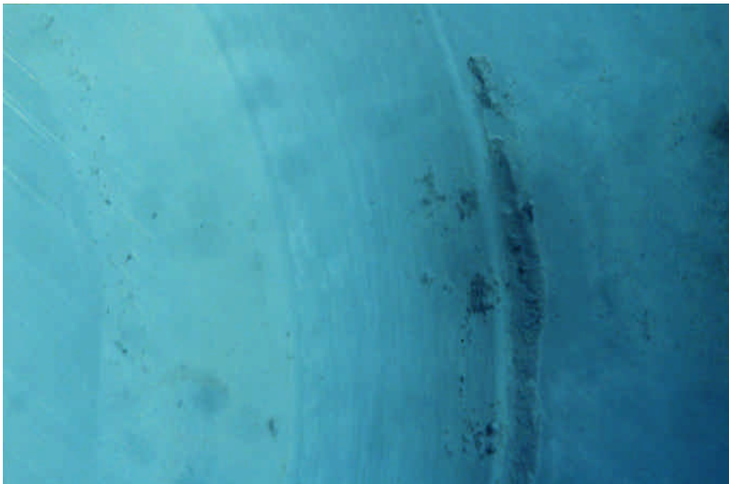
Figure 4.2.2.6 Filtered Ethyl-4-Amino Benzoate in Alumina A System, Test 42: Photomicrograph of Disk Wear Track (15.75 x)
