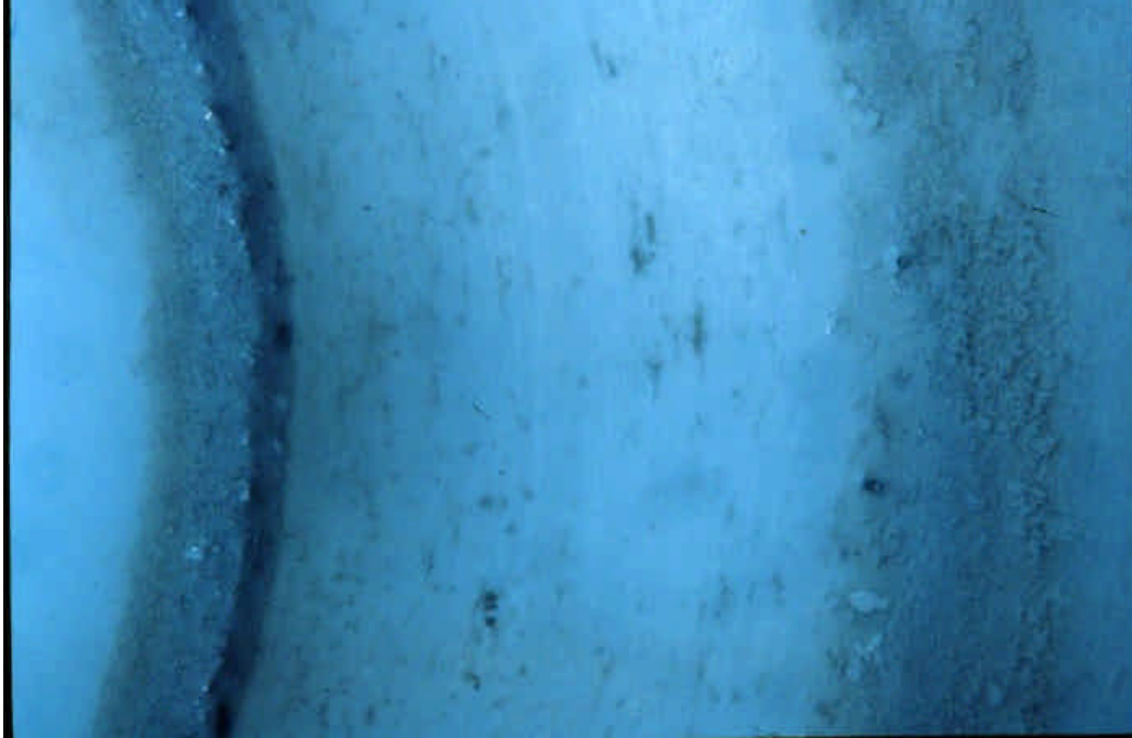
Figure 4.2.1.7 Alumina A System Reference, Test 41: Photomicrograph of Disk Wear Track (15.75 x)
