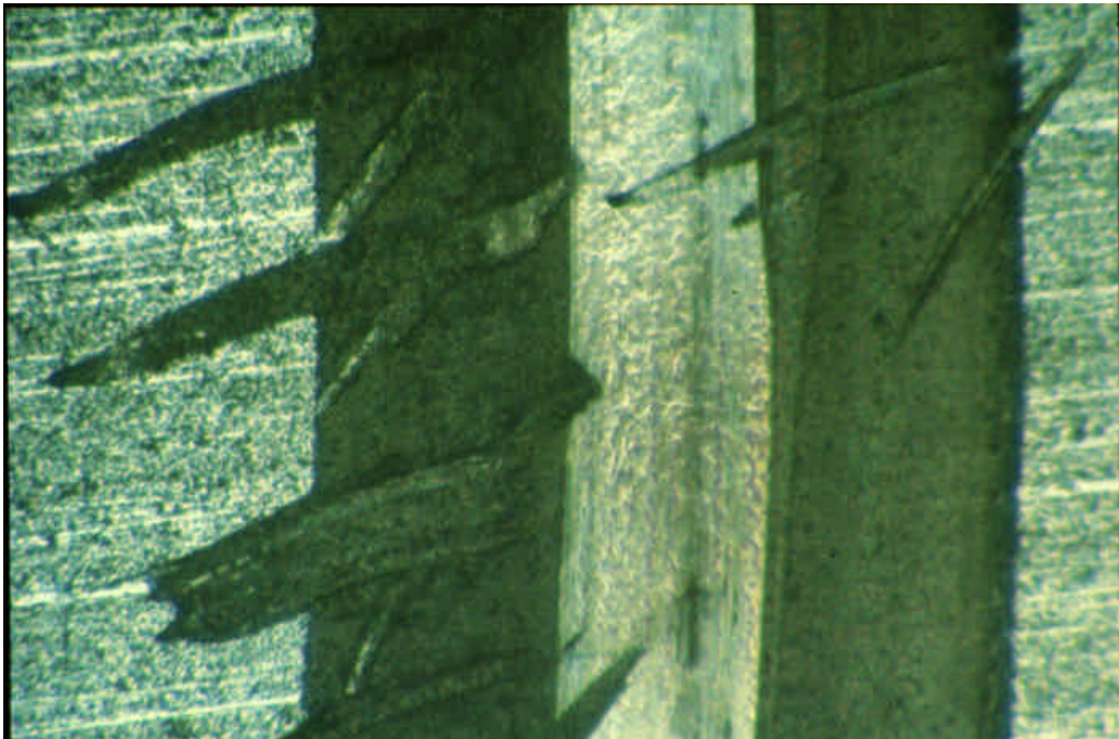
Figure 4.2.4.2 Caprolactam in Alumina A System, Test 30: Photomicrograph of Disk Wear Track (40 x)
