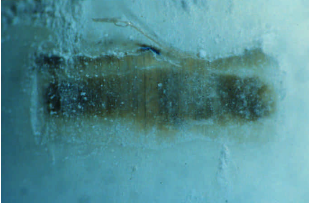
Figure 4.2.2.13 Methyl-4-Hydroxy Benzoate in Alumina A System, Test 34: Photomicrograph of Ball Wear Area (40 x)
