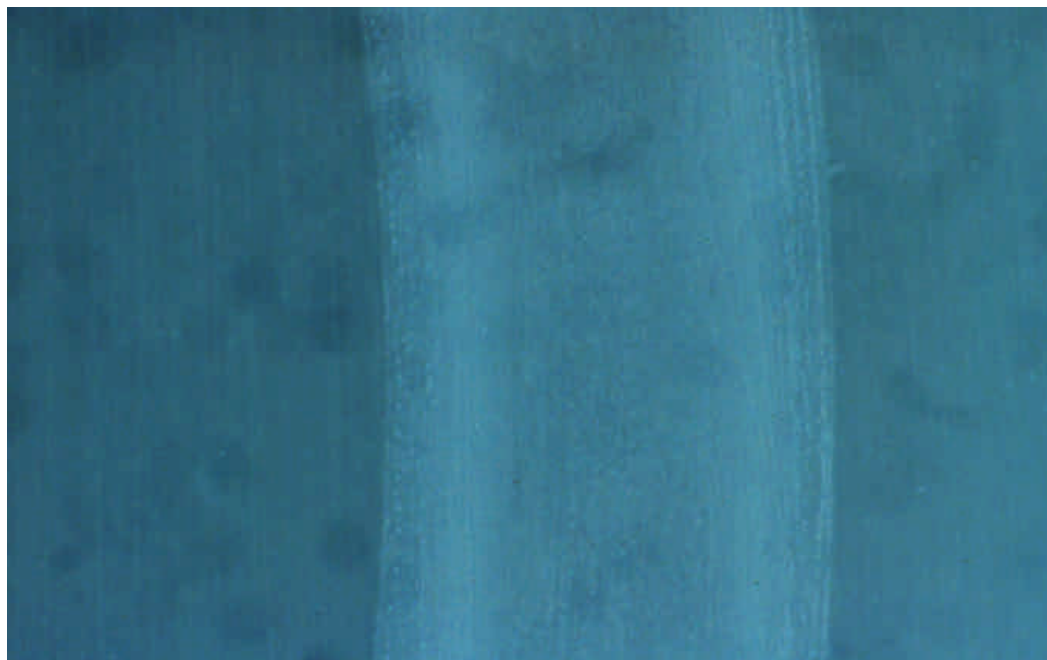
Figure 4.2.4.7 Filtered Caprolactam in Alumina A System, Test 43: Photomicrograph of Ball Wear Area (40 x).
