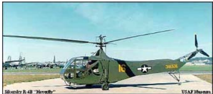
Figure 2.5 (b) First helicopter used in combat Sikorsky R-4 ( www.centennialofflight.gov )
