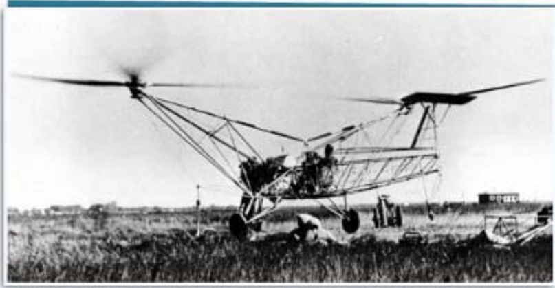
Figure 2.4: Focke's dual rotor helicopter ( www.eurocopter.com )
