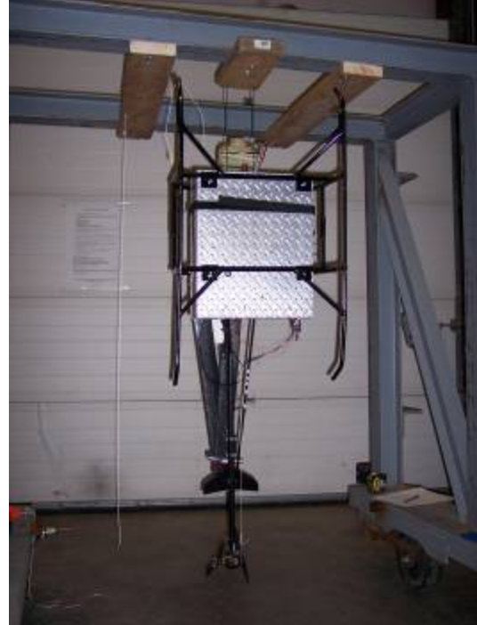
Figure A4b: Bifilar Pendulum Test
