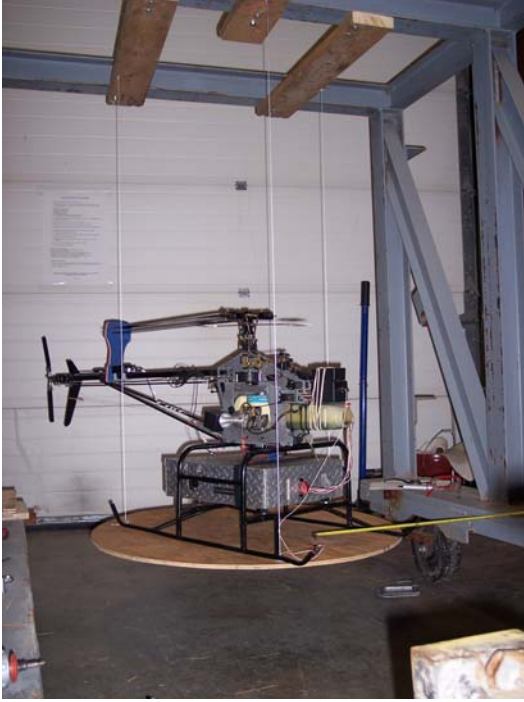
Figure A4a: Trifilar Pendulum Test
