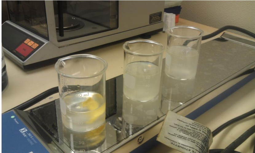
Figure 3. 7. Final Activity Test is being shown against Micrococcus Lysodeikticus . The solution will become visibly more clear and this uses the UV/VIS spectrophotometer to put a numerical number with the turbidity.
