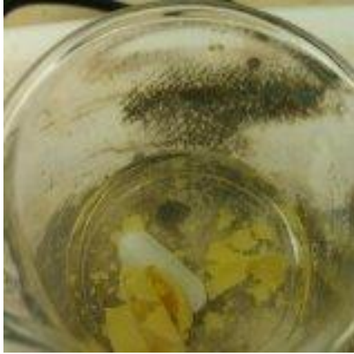
Figure 3. 10. Effect of pH Acidic film increased brittleness during final activity test.
