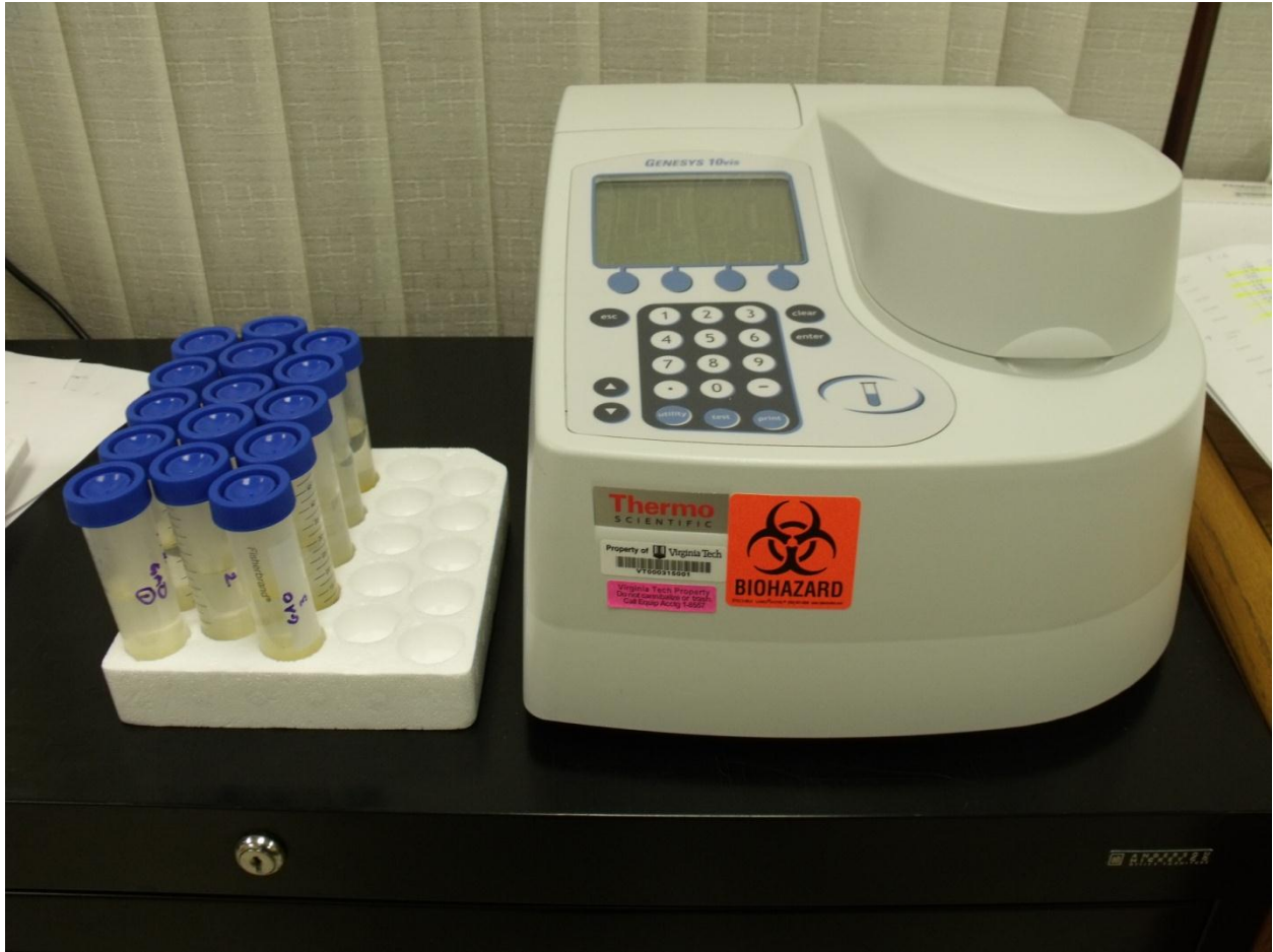
Figure 3. 2. The UV/VIS Spectrophotometer and samples during the release test.
