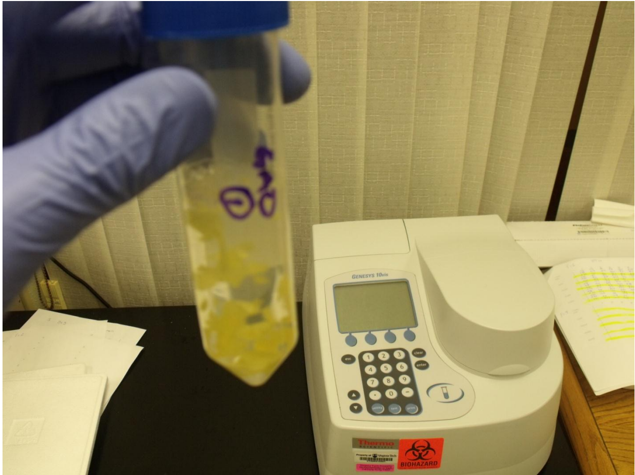
Figure 3. 13. Another example of the adjusted pH caused brittleness for the release test. When the sample was stirred prior to use the film would break down.
