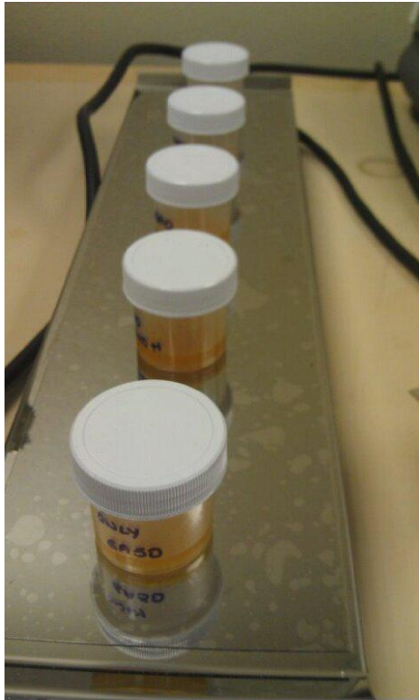
Figure 3. 3. Several different concentrations of Glutaraldehyde being mixed prior to casting under uniform conditions.
