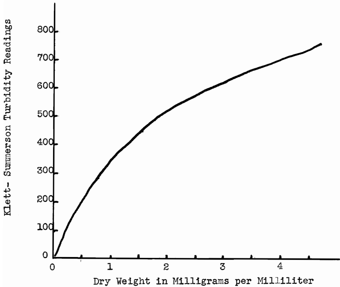
Figure 1. Turbidity - Dry Weight Curve for Rhizobium trifolii .
