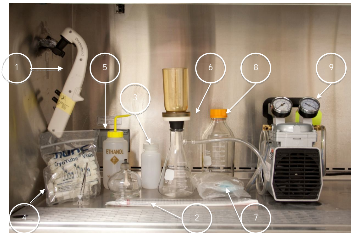
Figure 3-7. Experimental setup for filter capture.
