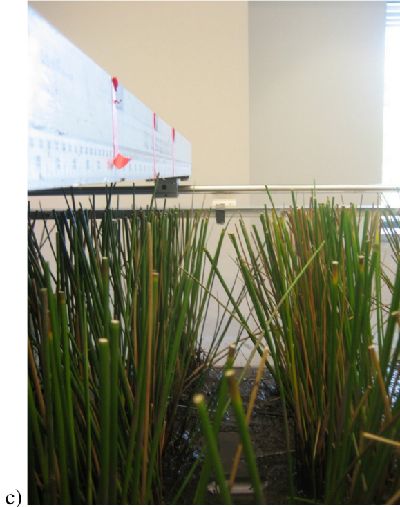
Figure 3. Images of flume set up a) overhead view of flume set up (not to scale) where the yellow dots are water surface level measuring locations, b) actual view of flume with gage set up, c) view of a cross section in the initial flume set up (12 cm diameter, 25 cm spacing)
