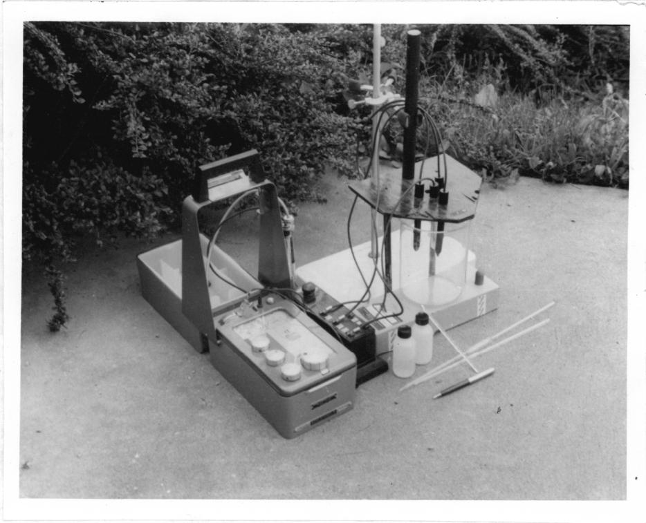
Plate 3. The Apparatus Used in the O-R Potential Determination
